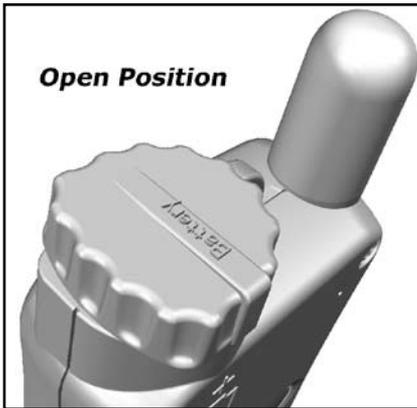
When the battery is first installed into the Pendant - you will hear an audible announcement of the battery status: "Battery is ok"; "Battery is low" or "Replace battery now". If the battery is fully discharged when you get your unit - you may not hear anything - at which point you will need to charge one of the batteries up overnight in the base charger before you will be able to use the system.
