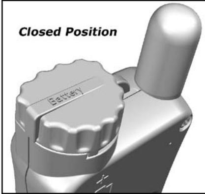
To install the battery - rotate the battery cap 90° counter-clockwise. Pull the battery cap straight up to remove. Install the battery with the positive side up facing the cap. Re-install the cap by aligning the cap as per the diagram to the left. Then push the cap back down and rotate 90° clockwise to lock in place.
