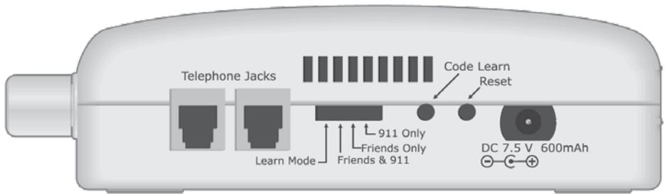
**Power Connection.** Simply plug in the AC Adapter in to the nearest electrical outlet. Plug the other end of the AC power adapter into the Base unit. You need to push the plug into the opening in the Base unit and twist 90° clockwise to lock in place. To remove in the future, simply rotate 90° counter-clockwise and pull outward.
