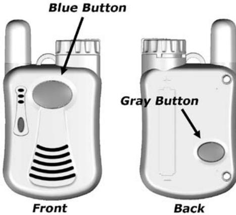
The Blue button on the front is the main button to push for a full second to initiate a call. Once this button is pushed the call proceeds forward to the 'Friends' list and or 911 depending on the slide switch setting on the back of the Base unit.
