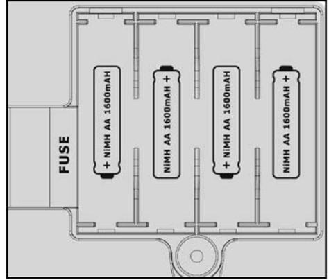
When you first get your unit - these batteries will probably be low, or even fully discharged - and will need to be charged overnight before being able to provide you the 24 hour battery back-up protection.
