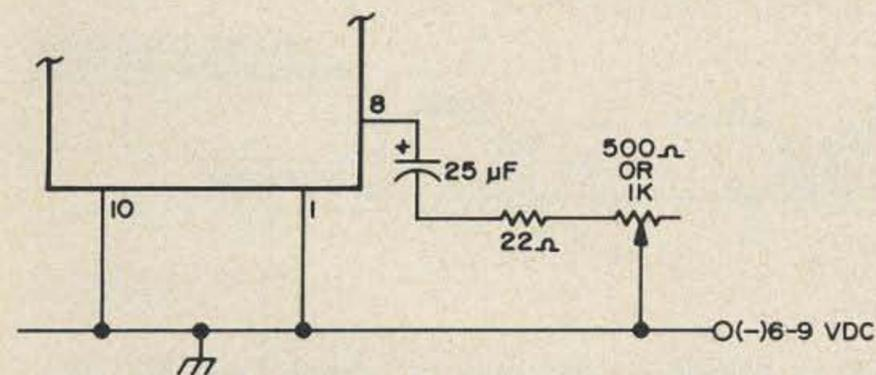
Fig. 3. Variable feedback control.
