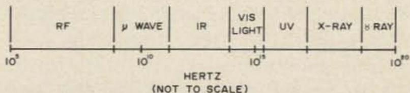
Fig. 1. Plot of electromagnetic spectrum shows energy distribution.
