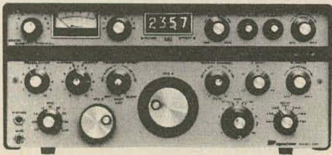
Quite frankly there is nothing with which to compare the CX7A. What else is there that has all modes 10 thru 160 meters with instant, no tuning band changing? With true break-in CW, a Pre I.F. noise blanker, R.F. clipping, and a built-in Keyer? With a separate receiver, wattmeter SWR meter, FSK shift, transmit offset and a freq meter digital counter?
