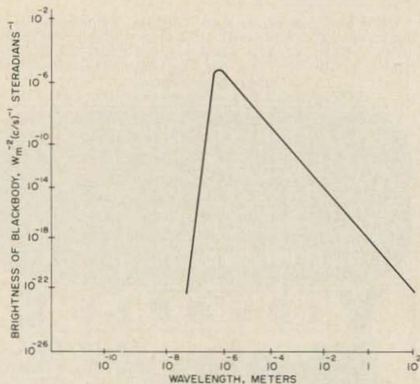
Fig. 3. Blackbody radiation curve for frequencies beyond rf portion of spectrum.
