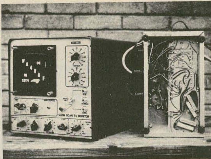
*The completed monitor. Underside view of power supply shows EKY circuit board that makes for simple construction.*
