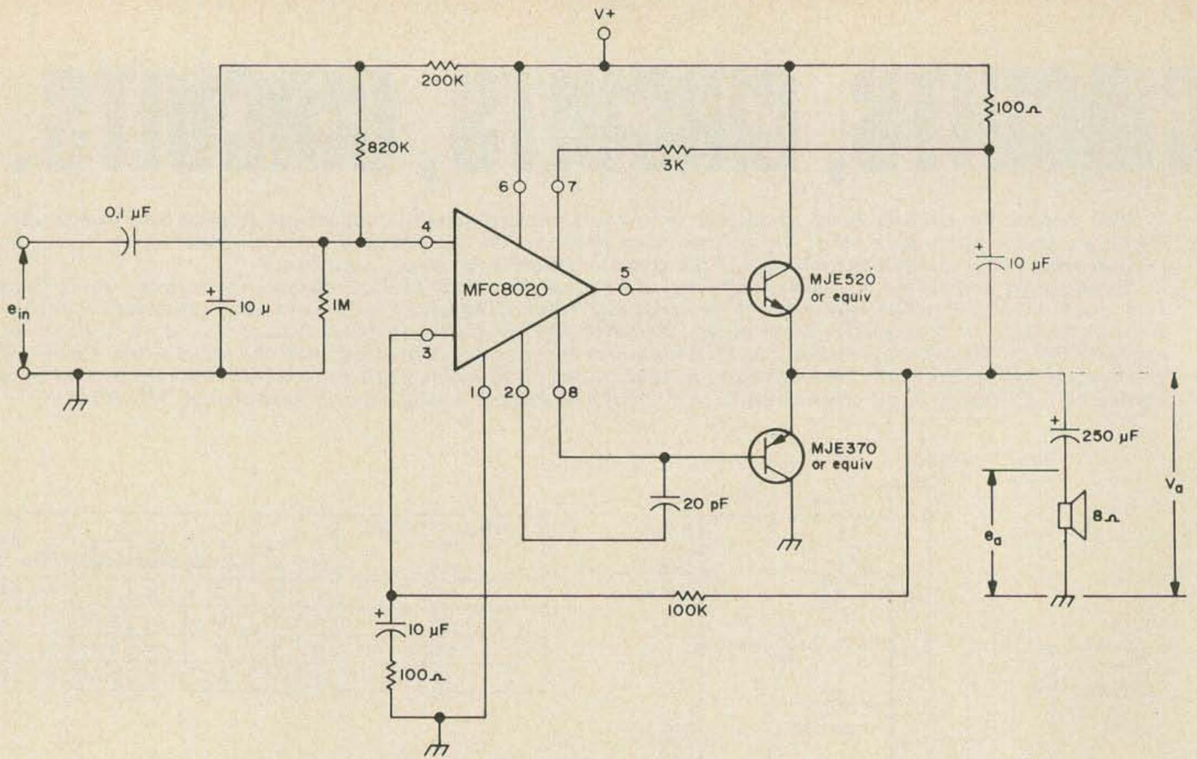
Typical application and test circuit (10-watt amplifier) using a Motorola MCF8020 class B audio driver silicon monolithic functional circuit. The MFC is designed as a preamplifier and driver circuit for complementary output transistors and will drive up to 15 watts output (4 ohm load). A application circuit courtesy of Motorola Functional Circuits Handbook.
