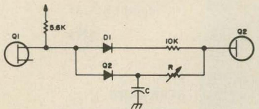
$D_1$  and  $D_2$  are 50 PIV 100AM diodes. The hold time is determined by the RC product. Typically, the C of  $200 \mu F$  and R of  $5K$  the hold time was 10 seconds. Values will differ from transistor to transistor and should be determined experimentally.
