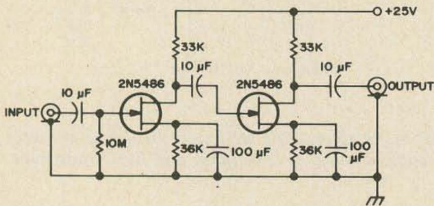
Low frequency preamp 1 Hz to 50 kHz, voltage gain 400, extremely low noise, all capacitances in  $\mu\text{F}$ , all resistors  $\frac{1}{2}\text{W}$ , transistors 2N5486. Circuit thanks to WA3EEC.
