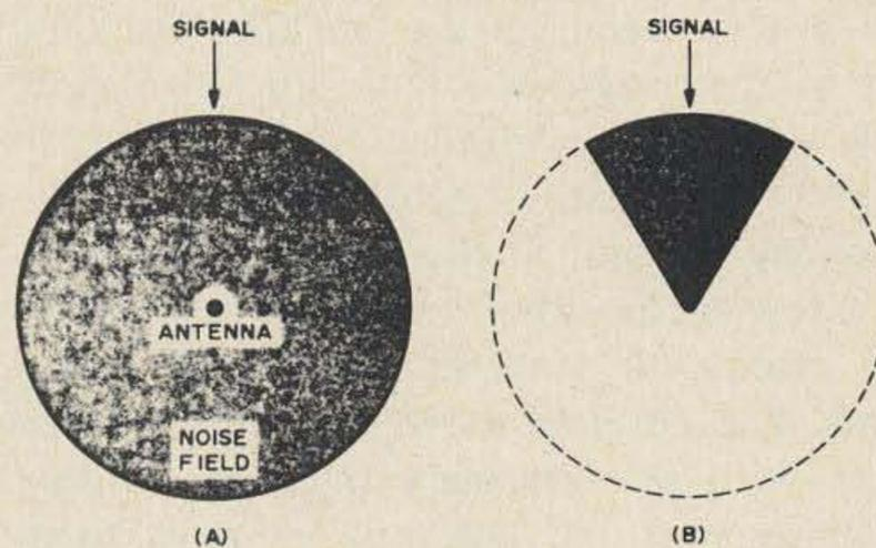
Fig. 3. The value of antenna directivity (B) for receiving purposes over an omnidirectional response (A) is that noise coming from directions other than that where a desired signal originates is discriminated against.
