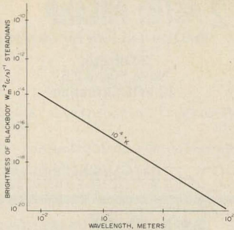
Fig. 2. Blackbody radiation, rf spectrum.
