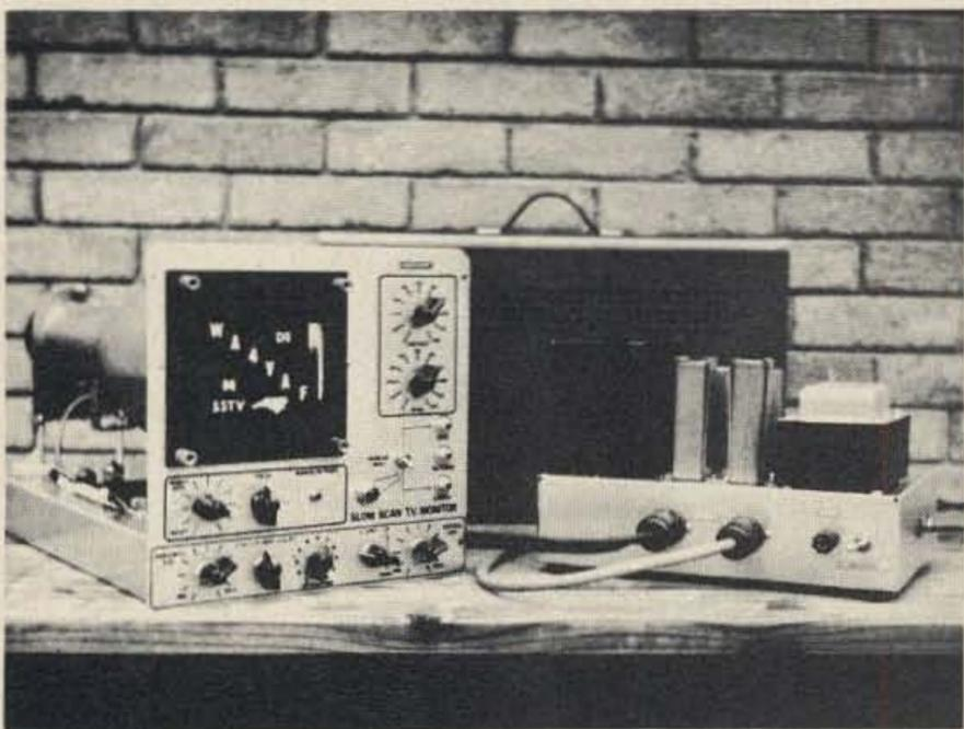
*The completed monitor with outboard power supply. Note the sub-mounted deflection board to the left and behind the panel. The cabinet which houses the monitor also has a neat carrying strap.*
