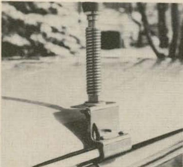
Here's new convenience in a rugged, all stainless mobile antenna gutter mount. The unit installs quickly with only a screw driver, is self-grounding and no holes are required in the auto body. Surprising signal results are received using a small spring and resonator only mounted on the 3/8-24 stud - no mast section is required. Also, it is easy to reach out the window and pull down the antenna for garages and other obstructions.
