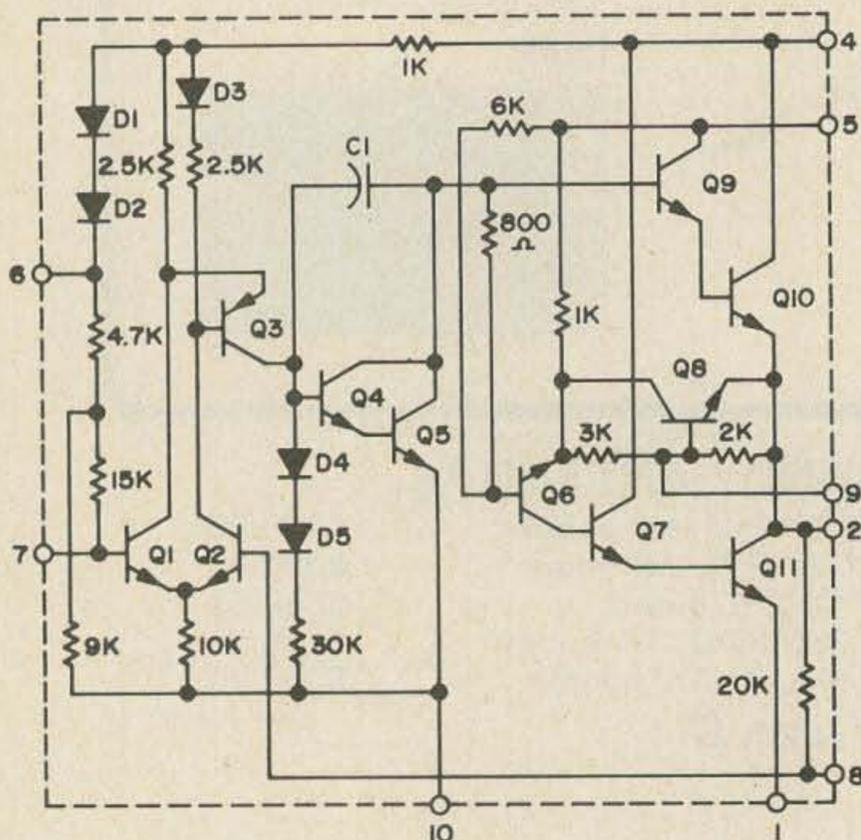
Fig. 1. Internal schematic of the TAA-300 Amperex audio amplifier IC.
