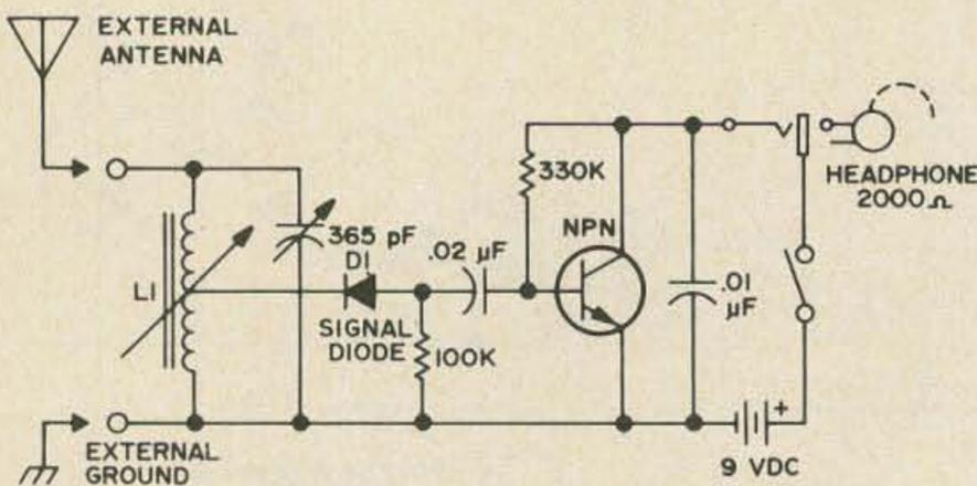
One-transistor radio. Works on local broadcast stations. Amuse the Jr. op. Circuit courtesy Calectro Handbook. L1 is a ferrite variable antenna coil (Calectro D1-841). D1 is and signal diode (Calectro K4-550).
