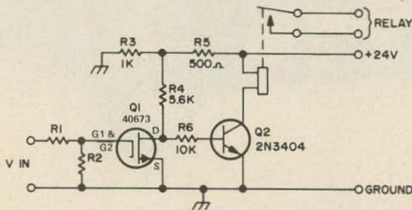
The first transistor stage utilizes a MOSFET with an extremely high input impedance. This feature allows connection to nearly any receiver with a minimum of loading. A negative going voltage of more than  $-3V$  is required to activate the COR. This voltage can normally be obtained from within the receiver squelch circuitry. With no received signal  $V_{in}$  should be approximately  $0V$ .
