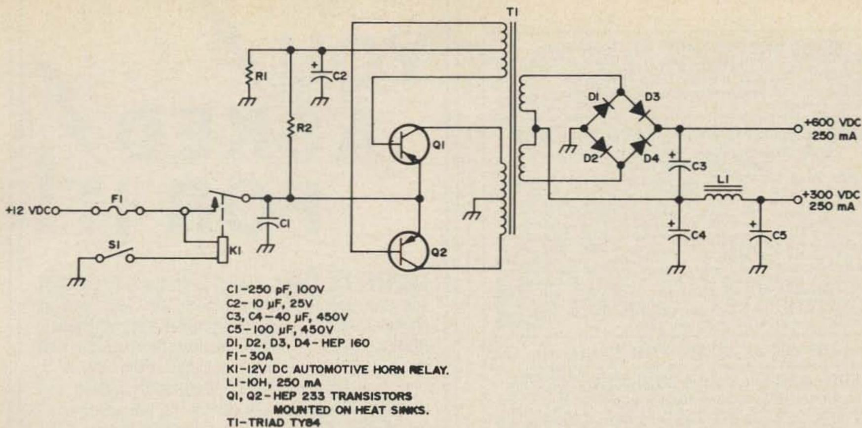
Mobile transceiver power supply (from The Keyer Ventura County ARC). 12V in, 600V @ 250 mA and 300V @ 250 mA out. Mount transistors on heatsinks.
