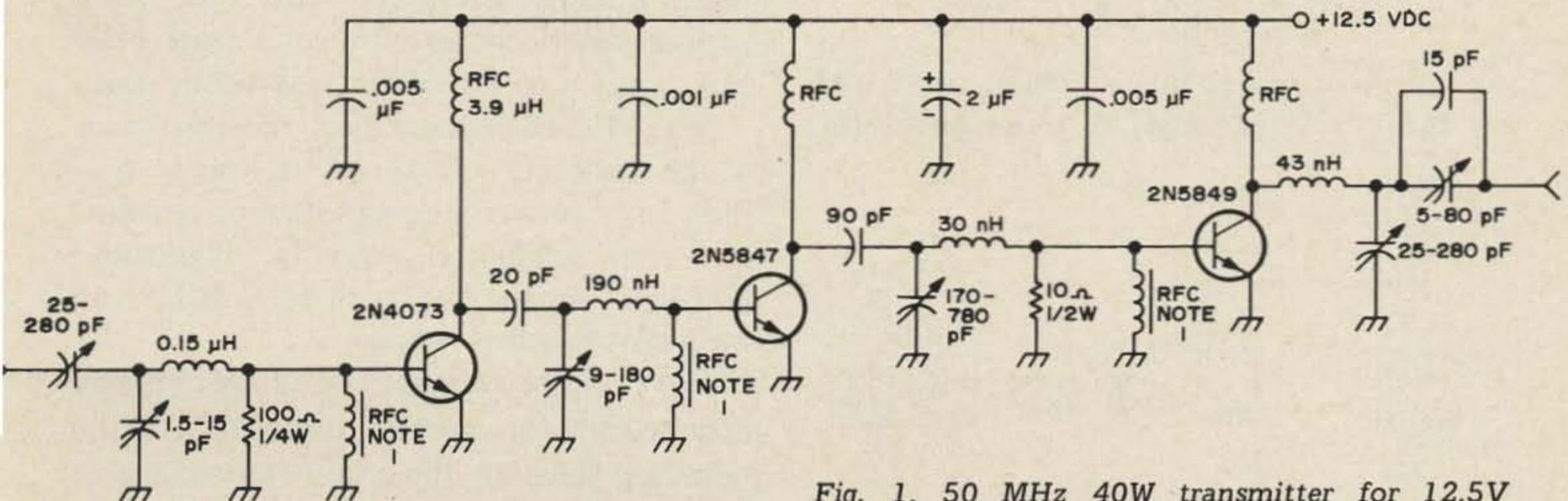
Fig. 1. 50 MHz 40W transmitter for 12.5V operation.
