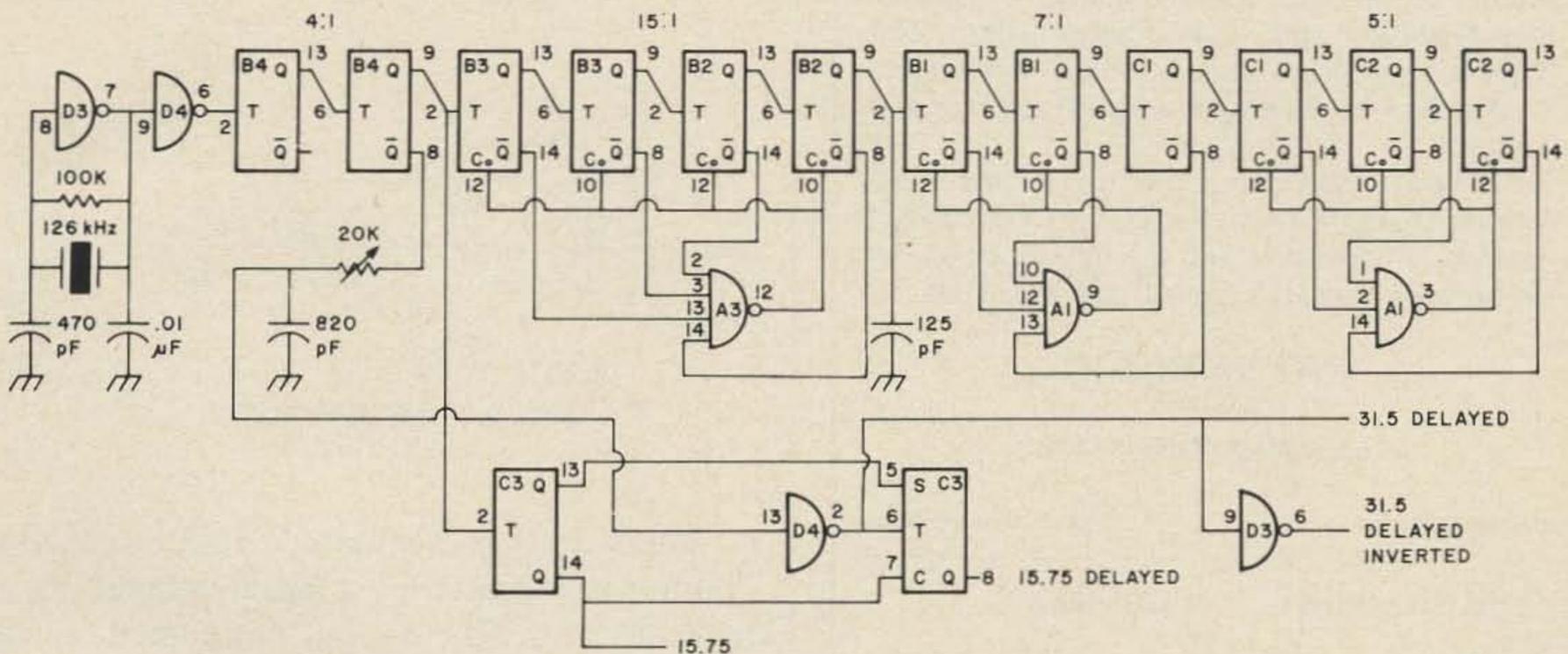
Fig. 2. Master oscillator frequency dividers.
