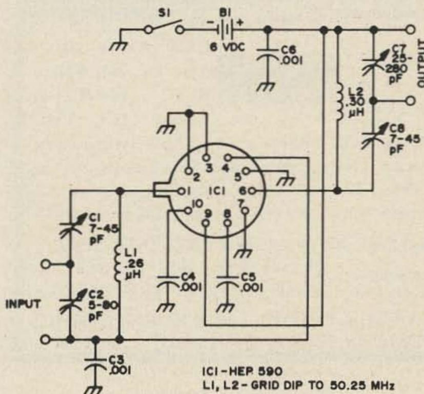
Six meter pre-amp with 30 dB of signal gain and 600 kHz bandwidth. The input and output impedances are matched. AGC may be added to pin 5. For FM use dip the coils to 52.5 MHz. Circuit from Motorola HMA-36, Radio Amateur's IC Projects, available free from Motorola, Dept. 73, Box 20924, Phoenix AZ 85034.
