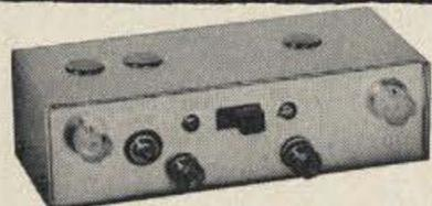
The Model 202 uses 2 of T.I.'s super low noise J-FETS in our special circuit board design which gives a minimum of 20 dB power gain at 450 MHz. Stability is such that you can have mismatched loads without it oscillating and you can retune (using the capped openings in the case) over a 15–20 MHz range simply by peaking for maximum signal. Available tuned to the frequency of your choice between 300–475 MHz. 4-3/8" X 1-7/8" X 1-3/8" aluminum case with BNC receptacles and power switch.
