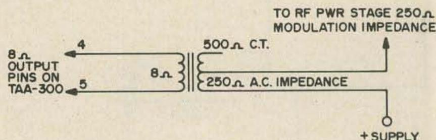
Fig. 5. Matching the output of the TAA-300 as a low power modulator using a small output transformer connected backwards.
