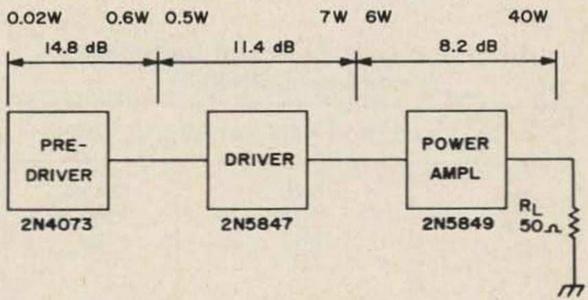
Fig. 2. Transmitter block diagram.
