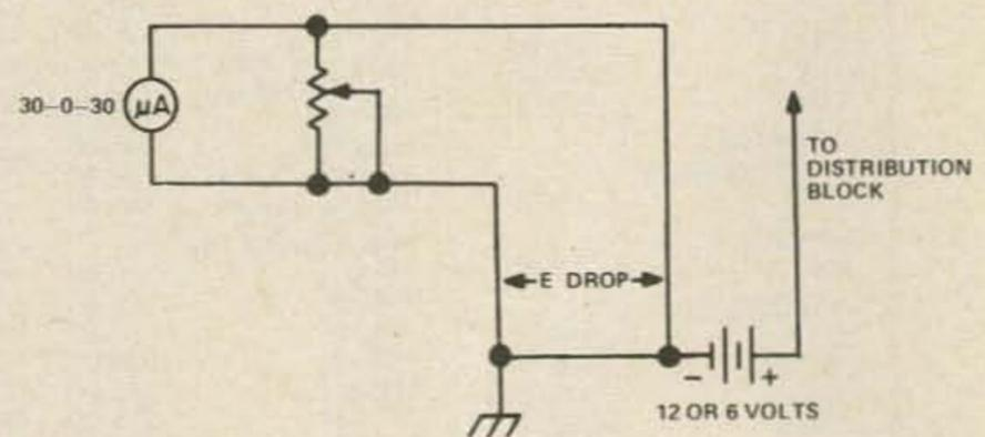
other accessories were turned on. An ancient wire wound, open type potentiometer was "scrounged" from the junkbox and placed across the microammeter terminals. This was adjusted until both meters read the same. The ammeter was then removed and the dc line closed.
