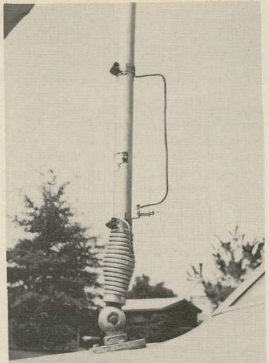
*The 47 dial light output indicator. This light bulb shows at all times positive indication of on-the-air and is all you need to tune and load the transmitter. The loop in this instance is completed by the antenna itself. Can also be used as a complete loop taped to the antenna.*
