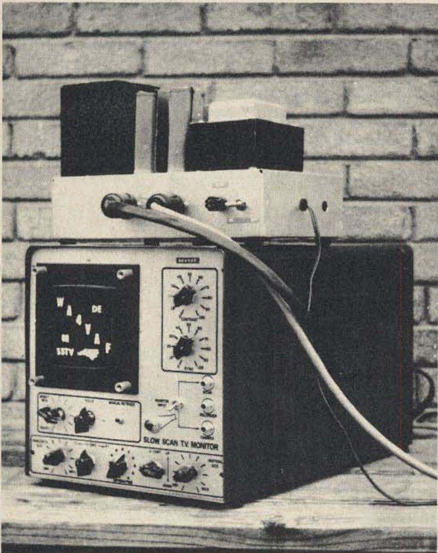
The completed monitor in store-bought cabinet. Outboard power supply on top. Panel was given a professional look by silk screening. Also note high-voltage wire enclosed in vinyl sheath for neatness.
