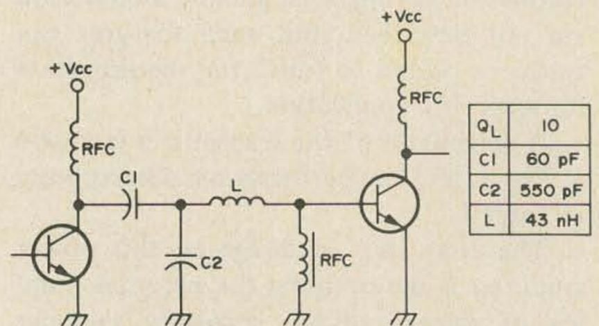
**Fig. 4. Driver/final interstage component values.**
