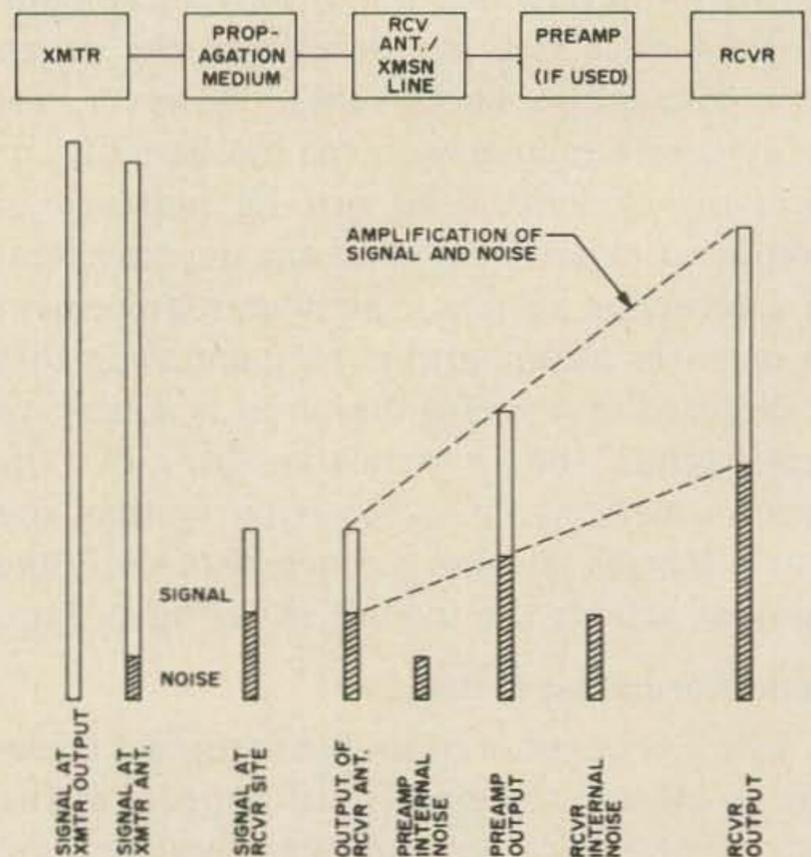
Fig. 2. The effect of noise and amplification at various steps in the transmitter output to receiver output chain.
