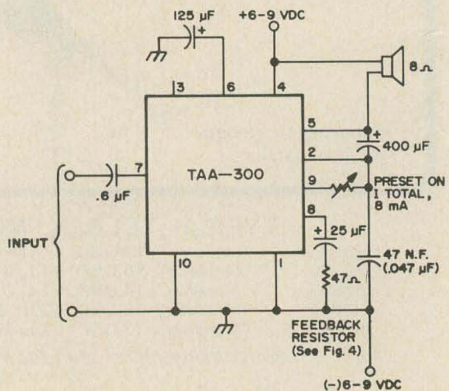
Fig. 2. External schematic of a complete audio amplifier using the TAA-300 IC.
