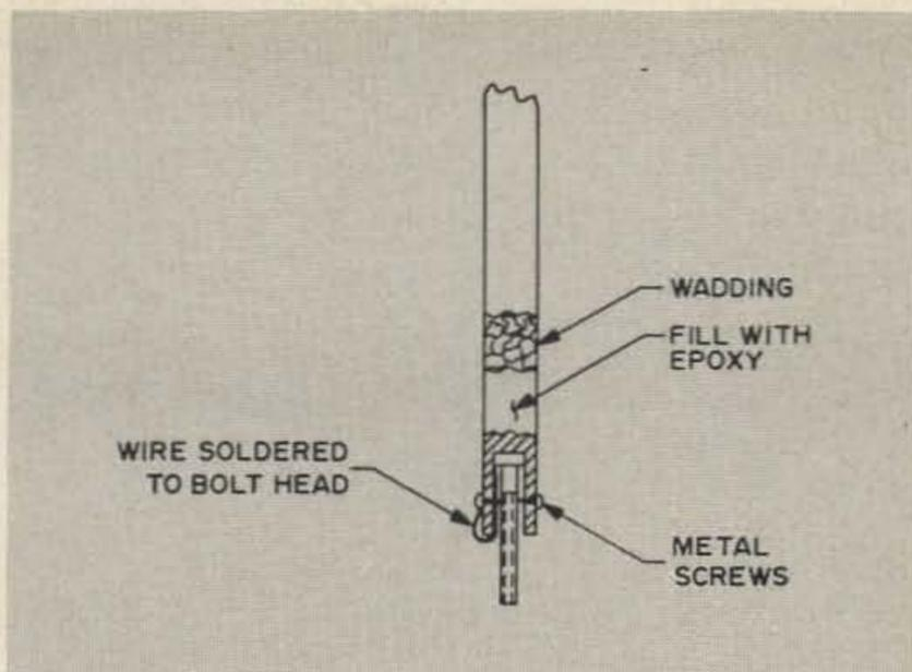
Or the plastic tube may be "splinted" to the base and temporarily "outside taped." Then the coil form and 6 in. of the base are filled with epoxy. The tip is placed in position and the whole thing hardens. This method is especially useful for the short coils, 40m and up.
