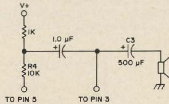
Motorola Functional Circuit MFC9000, in a typical application. This solid-state device is a 4-watt audio amplifier designed to provide the complete audio system in TV, radio and hi-fi equipment. Circuit courtesy Motorola MFC Handbook.
