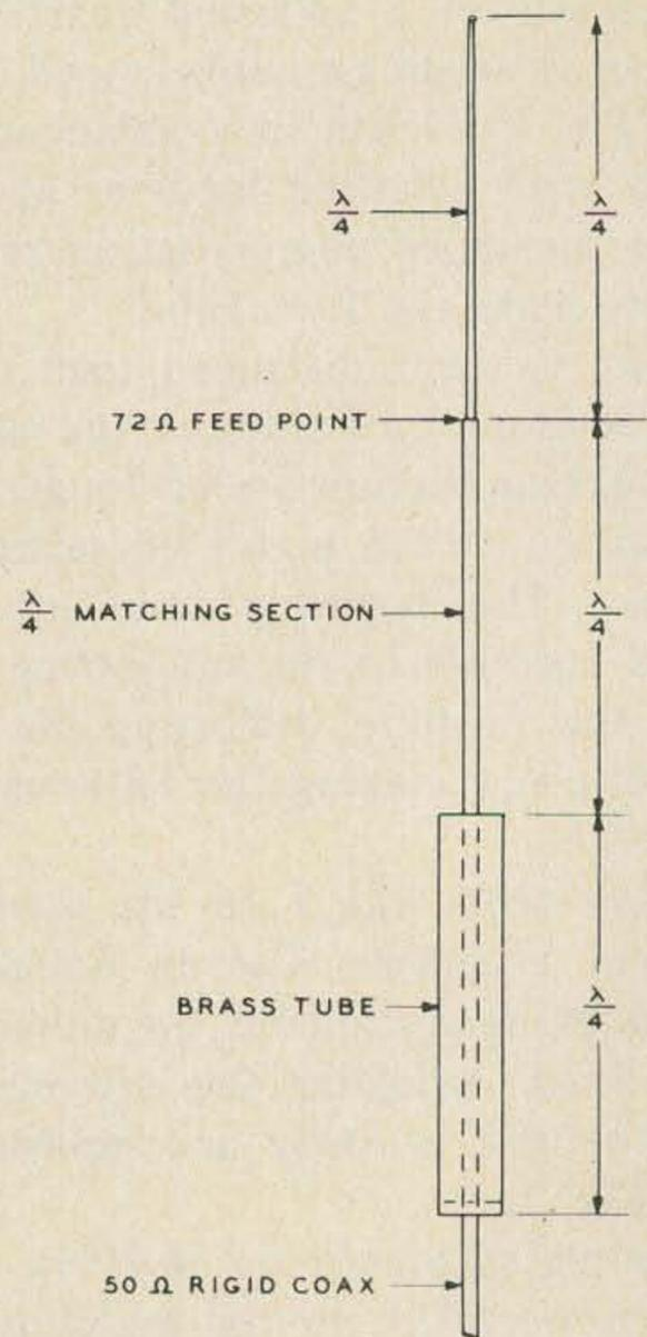
Fig. 4. Reynolds modified sewerpipe antenna.
