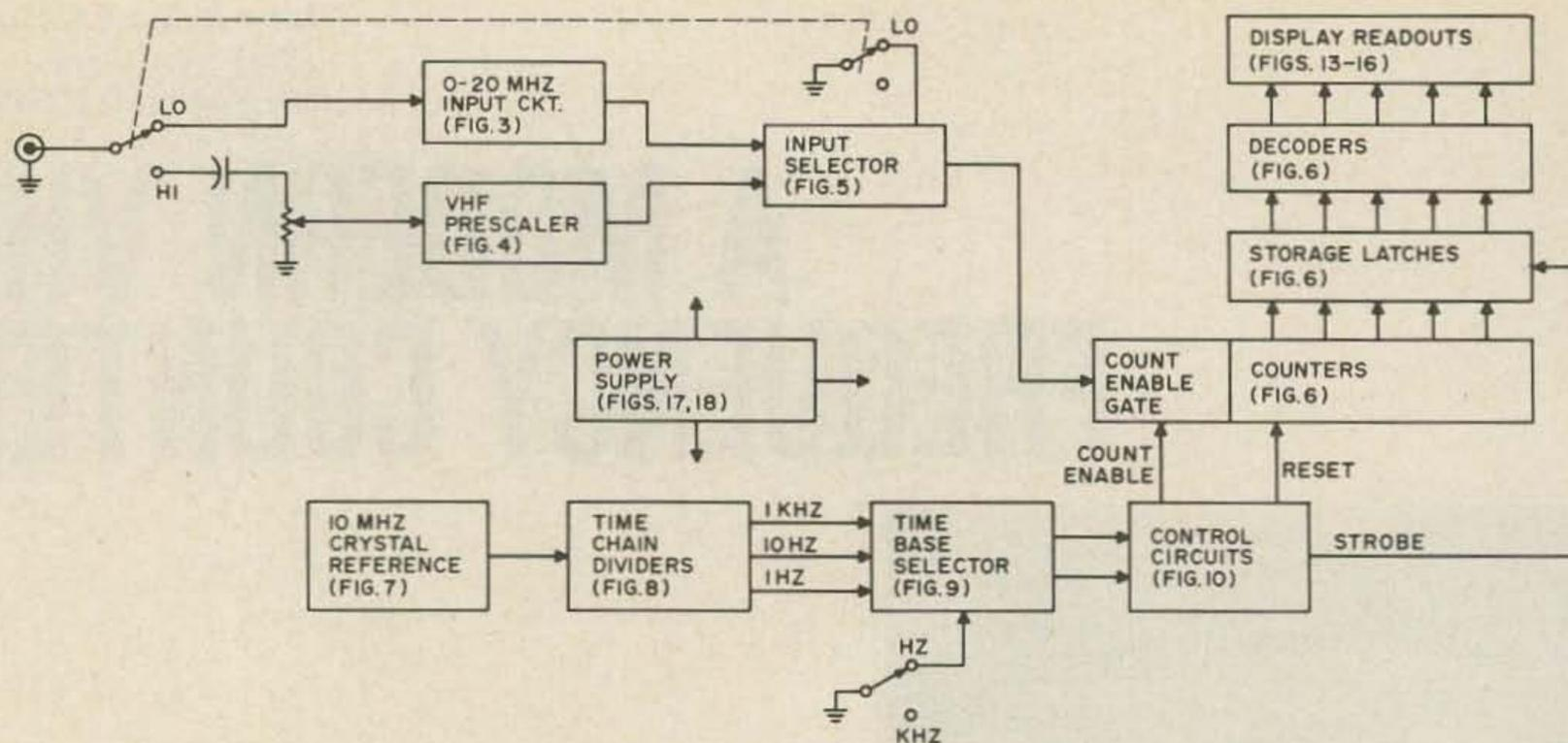
Fig. 1. Counter block diagram.
