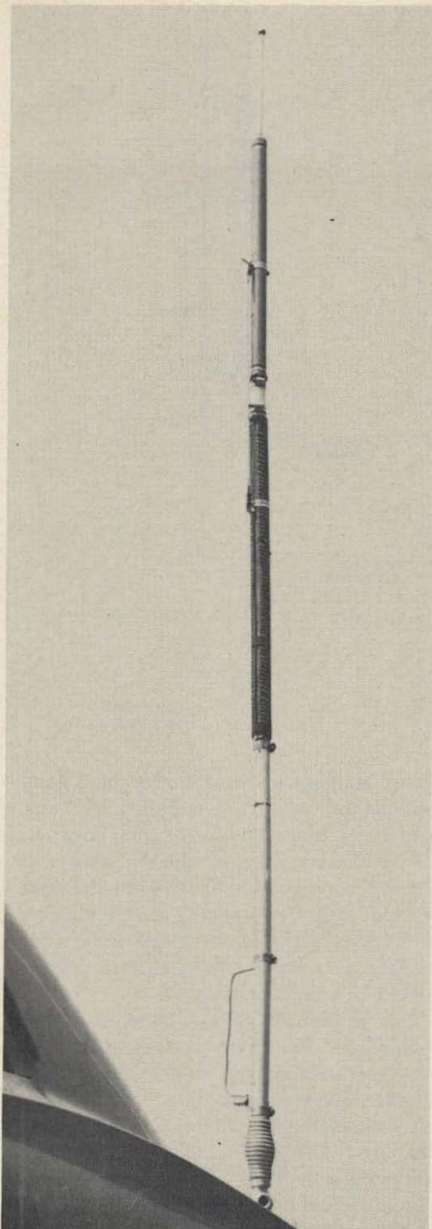
*Antenna installed on 67 Chev. Used with Motorola SB3 Rig.*
