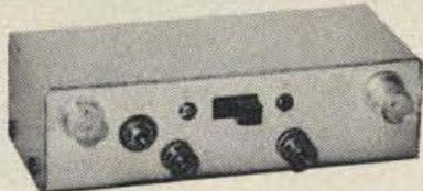
35 dB power gain, 2.5–3.0 dB N.F. at 150 MHz, 2 stage, R.F. protected, dual-gate MOSFETS. Manual gain control and provision for AGC. 4-3/8" X 1-7/8" X 1-3/8" aluminum case with BNC receptacles and power switch. Available factory tuned to the frequency of your choice from 5 MHz to 350 MHz with approximately 3% bandwidth. Up to 10% B.W. available on special order.
