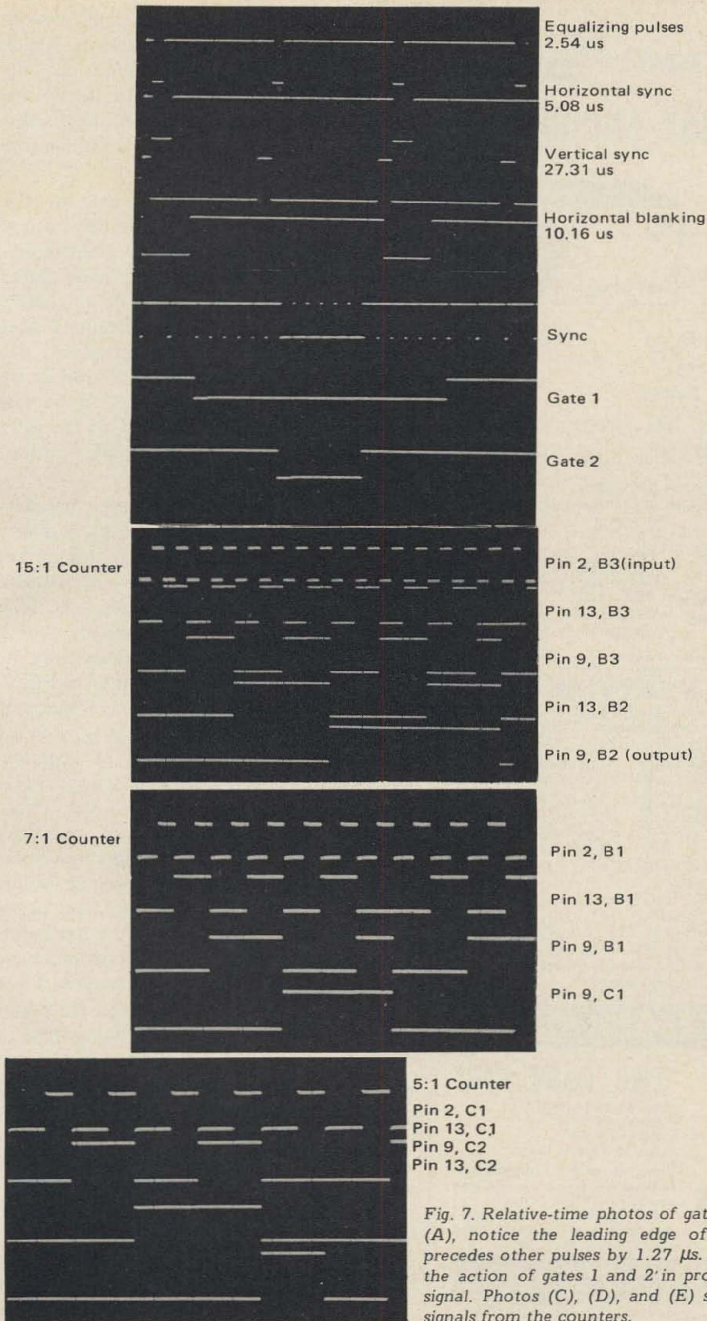
Fig. 7. Relative-time photos of gating functions. In (A), notice the leading edge of blanking pulse precedes other pulses by 1.27  $\mu$ s. Photo (B) shows the action of gates 1 and 2' in producing the sync signal. Photos (C), (D), and (E) show the output signals from the counters.
