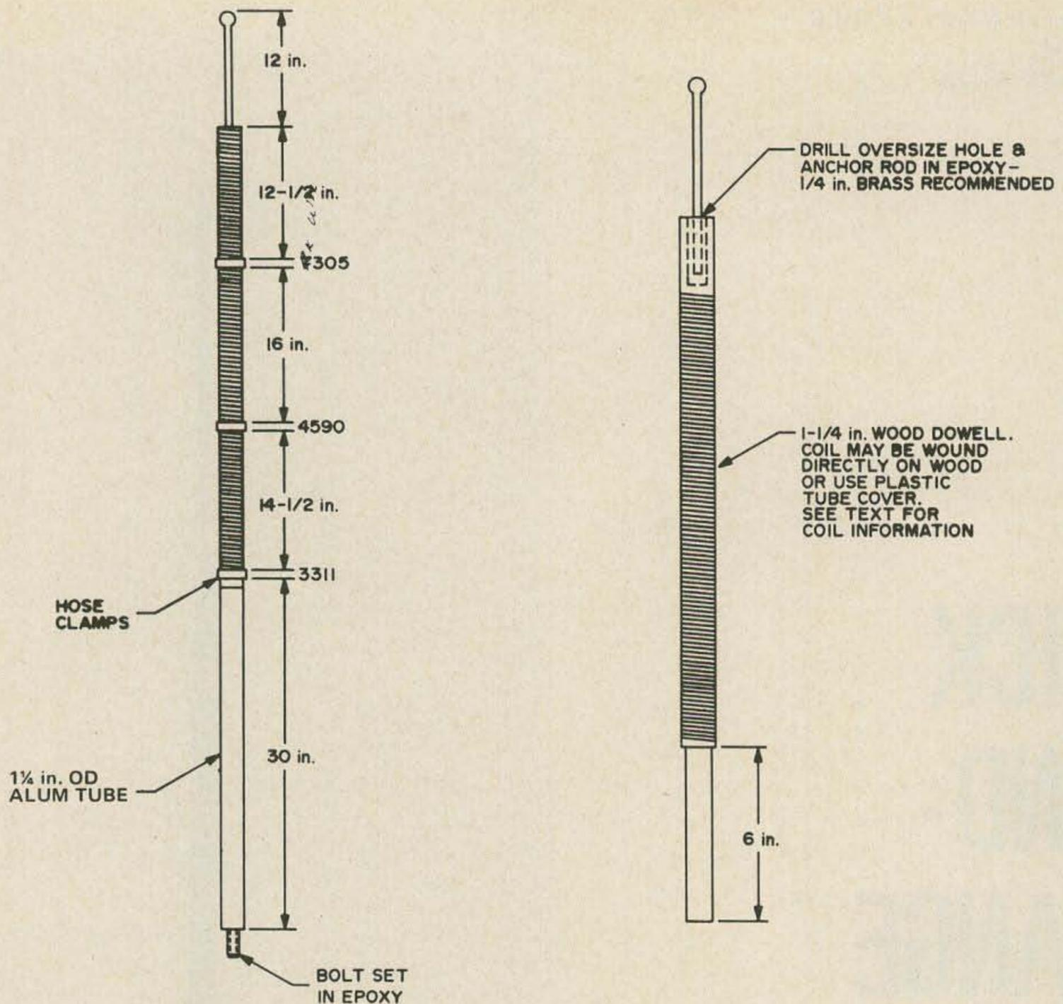
It was temporary, being wound on a bamboo fishing pole. Taps were brought out, with many trials and more errors; however, this temporary antenna worked so well it literally stayed on the car until the base "rotted" off. Had I coated the fishing pole with epoxy, I would probably still be using it. This antenna was wound with plastic-coated 20-gauge stranded wire.
