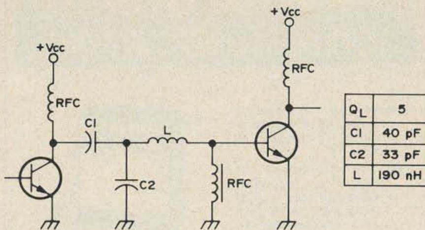
Fig. 5. Predriver/driver interstage component values.
