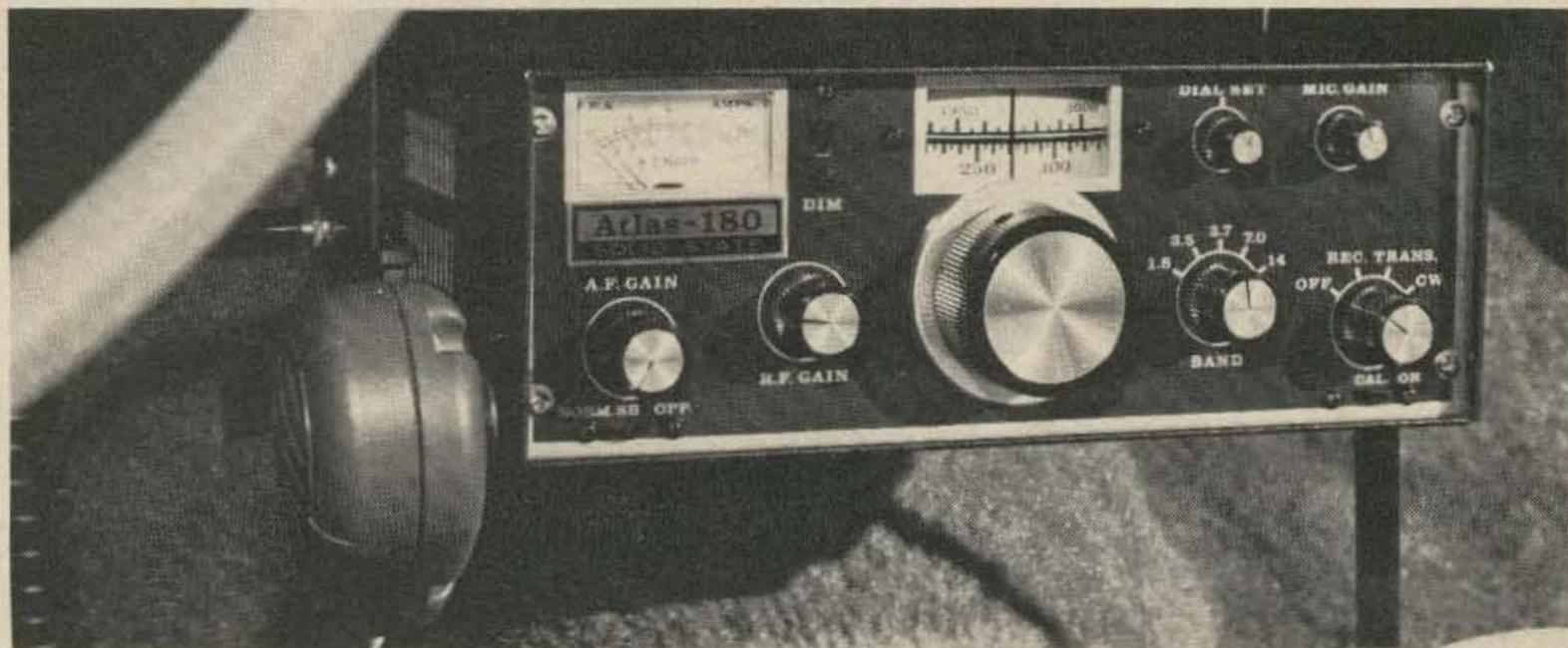
WITH THIS MOBILE RIG YOU CAN QSO all over the state, across the country, and even work intercontinental DX, right from the driver's seat, and without the aid of a repeater! Only a little bigger than a 2 meter FM rig, the Atlas-180 is an all-solid-state SSB-CW Transceiver that covers 4 bands, 20-40-80, and 160 meters, with a power input rating of 180 watts, and sells for only \$479. See your Atlas dealer for complete details, or write us for a brochure and dealer list.
