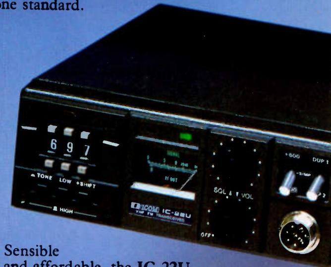
Sensible and affordable, the IC-22U offers simplicity with ease of operation. Easy to use push buttons for up and down tuning. 800 channels at the push of a button. 4 MHz coverage. EX-199 optional remotable frequency selector.
