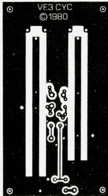
Fig. 11. One-stage preamp board PCB layout.
