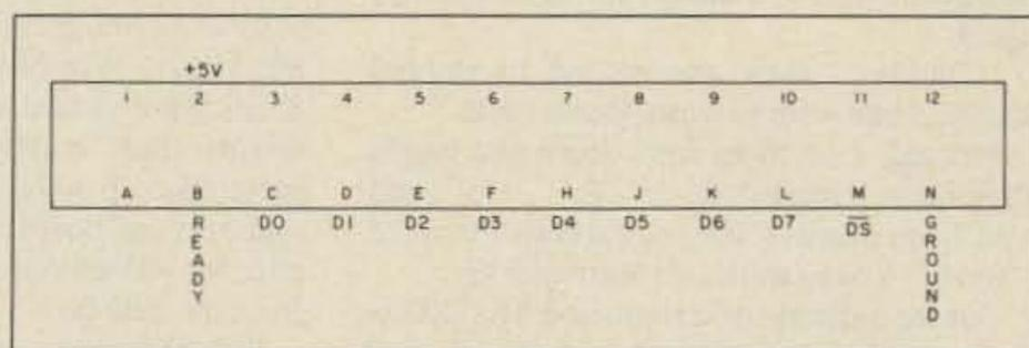
Fig. 3. Rear-view connector to VIC-20 user I/O port.
