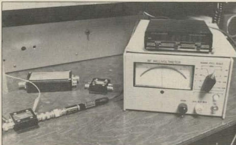
Photo B. 220VDA preamplifier under test with Ramsey counter and Boonton 92 millivoltmeter.
