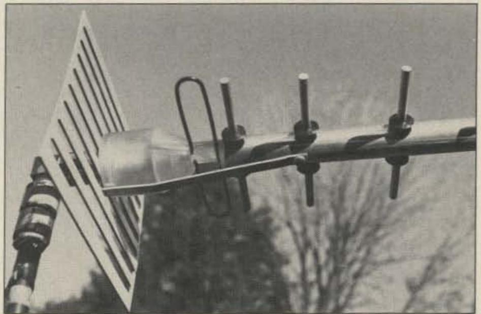
Photo B. The driven element and reflector assembly up close. The balun is made from miniature hardline.
