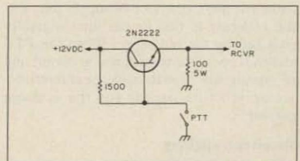
Fig. 4. Circuit for switching 12 V dc to the receiver section.
