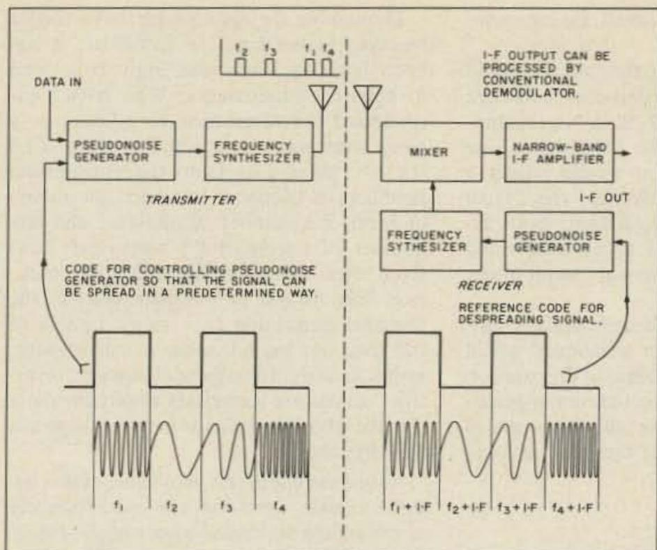
Fig. 4. Simplified block diagram of the spread-spectrum communications link. This "frequency-hopping" system transmits and receives over a bandwidth that is many times that of the data. The actual spectral distribution of the signal is controlled by a predetermined code that must be the same for both transmitter and receiver.
