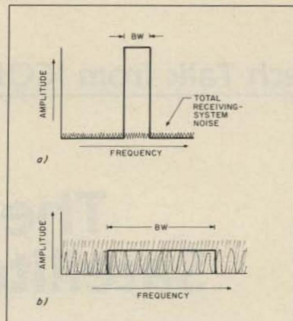
Fig. 3. Comparison between conventional and spread-spectrum signals. The power density of the spread-spectrum signal is very small compared to conventional modulation formats; indeed, the spread-spectrum signal may even be below the noise floor of the receiving system. (a) An ordinary signal in the rf spectrum. Here, the bandwidth may be about 3 kHz. (b) A spread-spectrum signal. Bandwidth could be a hundred thousand times wider than the bandwidth of the ordinary signal.
