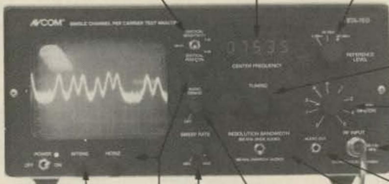
**TUNING** allows you to select the center frequency and moves the display "window" up or down the spectrum being displayed.
