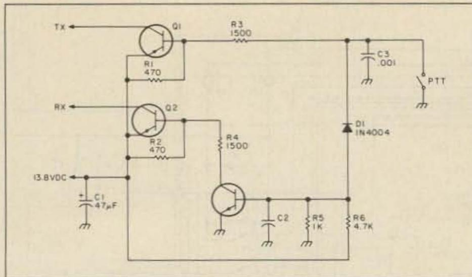
Fig. 5. Complete TX/RX voltage switching circuit.
