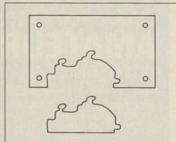
Fig. 1. Patch for a damaged circuit board.
