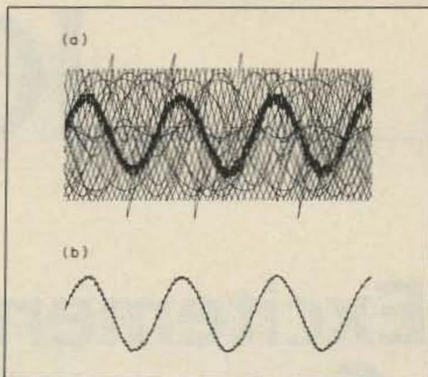
Fig. 2. Recovery of a signal from a background of noise. (a) The commonly encountered signal-plus-noise format. (b) The extracted signal after processing by filtering, integration, or correlation techniques.
