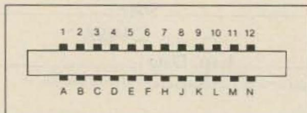
Fig. 2. User I/O port, rear view.
