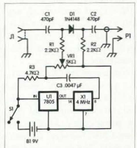
**Fig. 1.** Schematic diagram of the offset attenuator.
