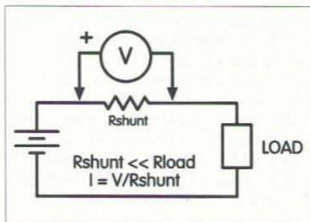
Fig. 1. Using a shunt to measure current.
