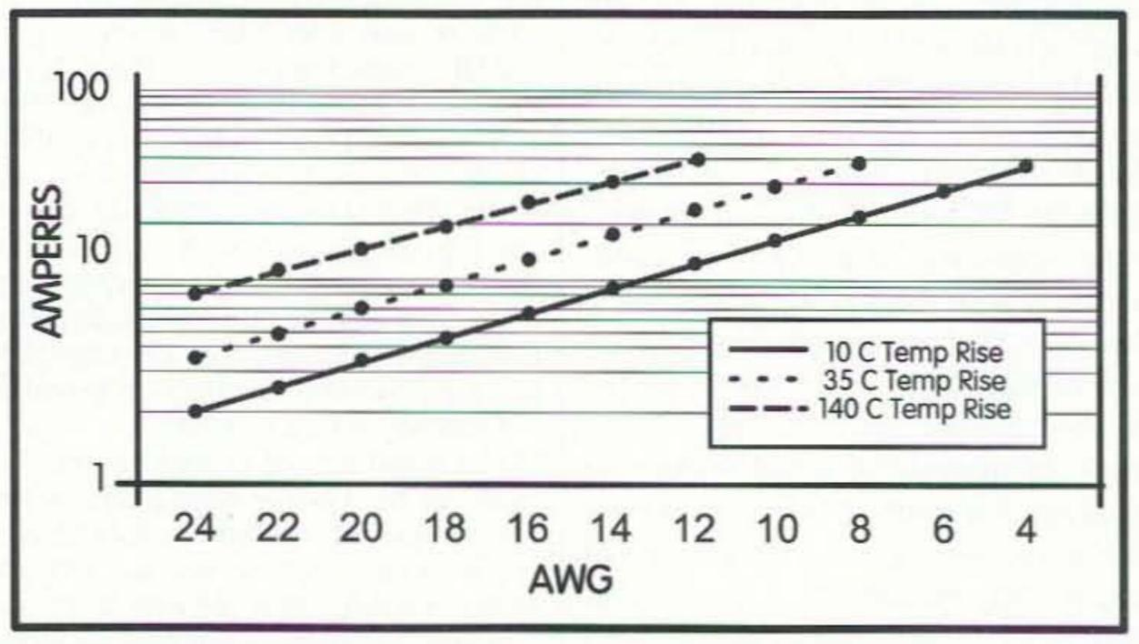
Fig. 2. Current-carrying capacity of wire.
