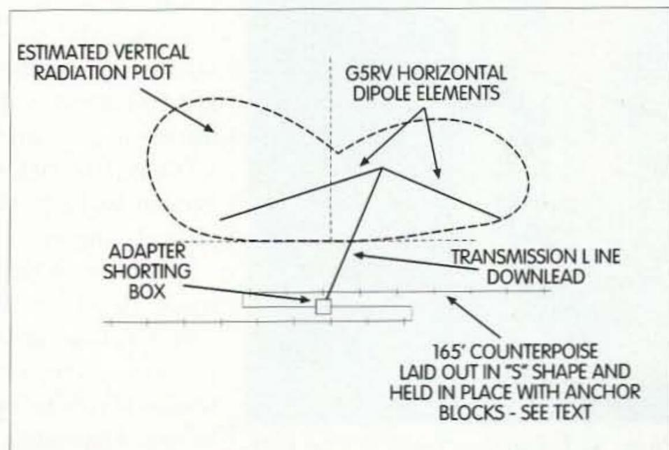
**Fig. 2.** AD1B's modification to the popular G5RV HF dipole antenna to permit contest weekend operation on 160 meters.
