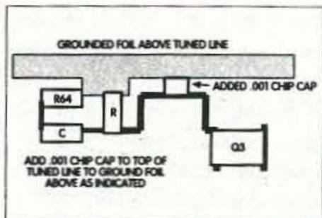
**Fig. 3.** Modification to VCO circuit on synthesizer board to convert original VCO frequency from 800 MHz range to 1152 MHz. Add .001  $\mu$ F chip capacitor from top of printed inductor to ground. This bypass capacitor increases VCO frequency from 700 MHz to 1200 MHz.
