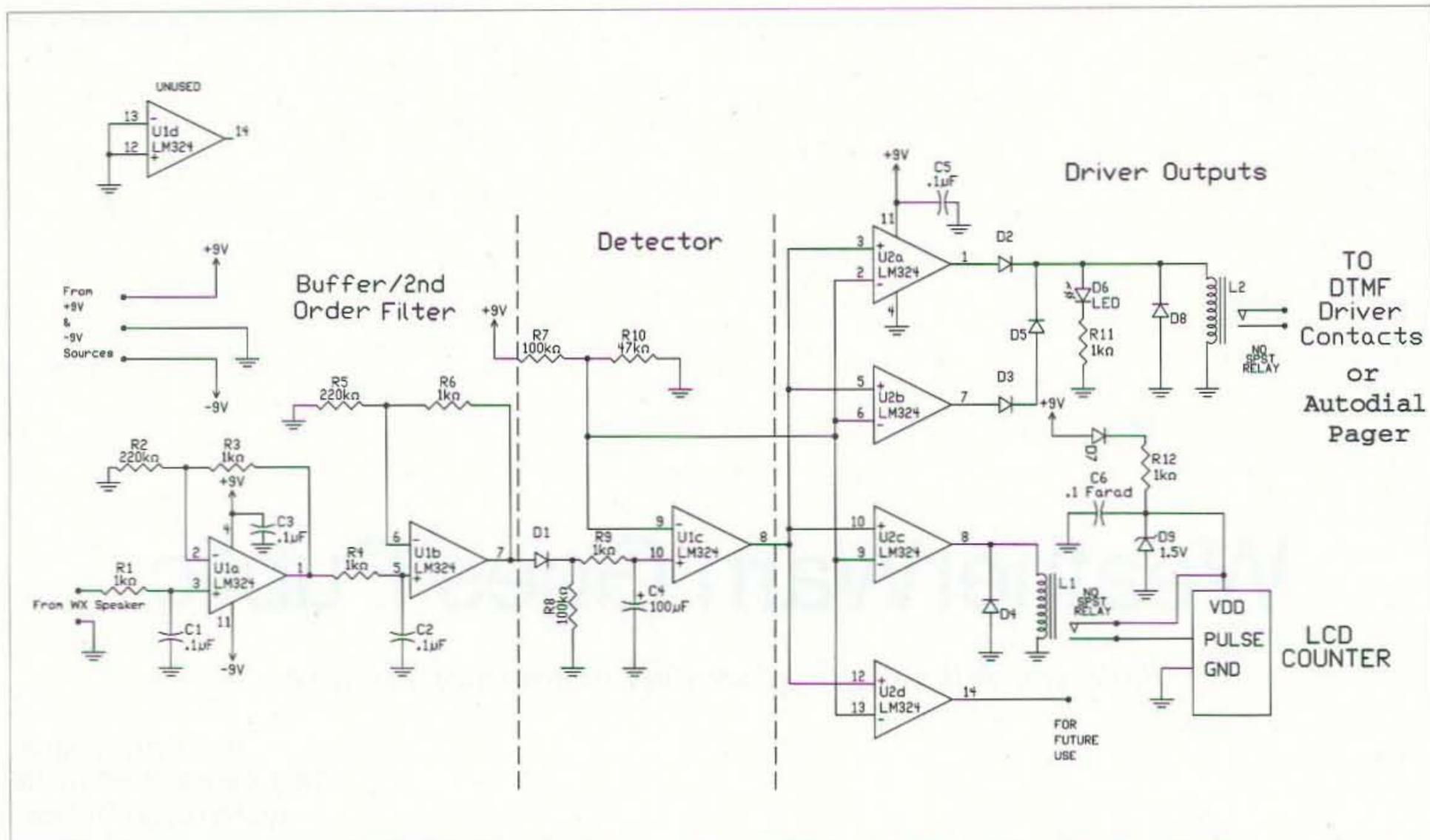
Fig. 1. WeatherWarn interface schematic. Unless otherwise specified, all diodes are 1N4007, all resistors are  $\pm 5\%$ , and all capacitors are +16 V.
