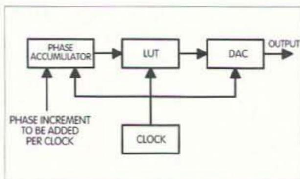
Fig. 2. Block diagram of a basic DDS with the major functions shown.
