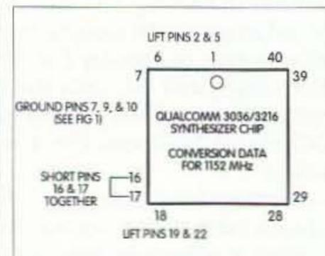
Fig. 2. Pin-for-pin conversion of Qualcomm synthesizer to 1152 MHz. Leave all other pins as they are.
