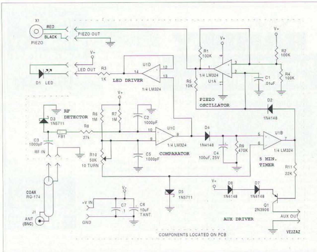
Fig. 1. Circuit diagram for the RF Sensing Alarm.
