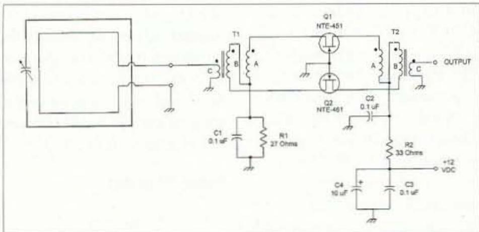
Fig. 8. Push-pull JFET preamplifier.
