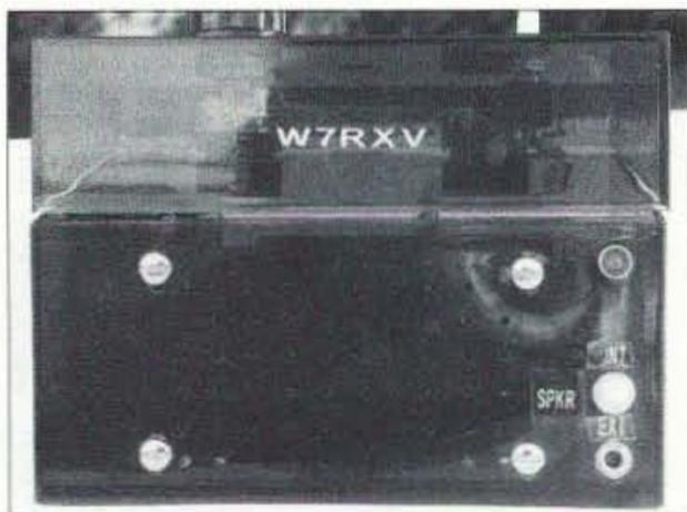
**Photo C.** Metronome in better-grade card file box, showing results of taping graph paper to box for layout. LED1, upper right, flashes in step with tocks, or silently if INT/EXT speaker switch is set for EXT and no external speaker is connected.
