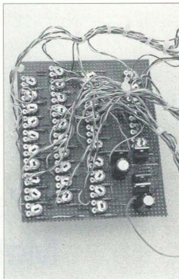
**Photo E.** Overall view of board in deluxe model. The regulator and pulse generator are on the lower right side of the board, while the fixed resistors and their trimmers take up the rest of the space.
