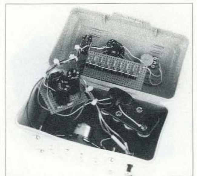
**Photo B.** Inside a basic, bare-bones, blue-box metronome with perfboard construction and eight preset tempos. A close look at the battery pack will show a tap, one way to get the correct voltage to Q1 and Q2 before trying the regulators. This does work while the batteries are fairly fresh. However, it does not give the best repeatability—sometimes that is a consideration.
