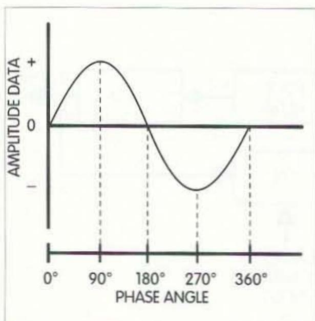
Fig. 3. The waveshape of the output signal from a DAC as mapped in the LUT.
