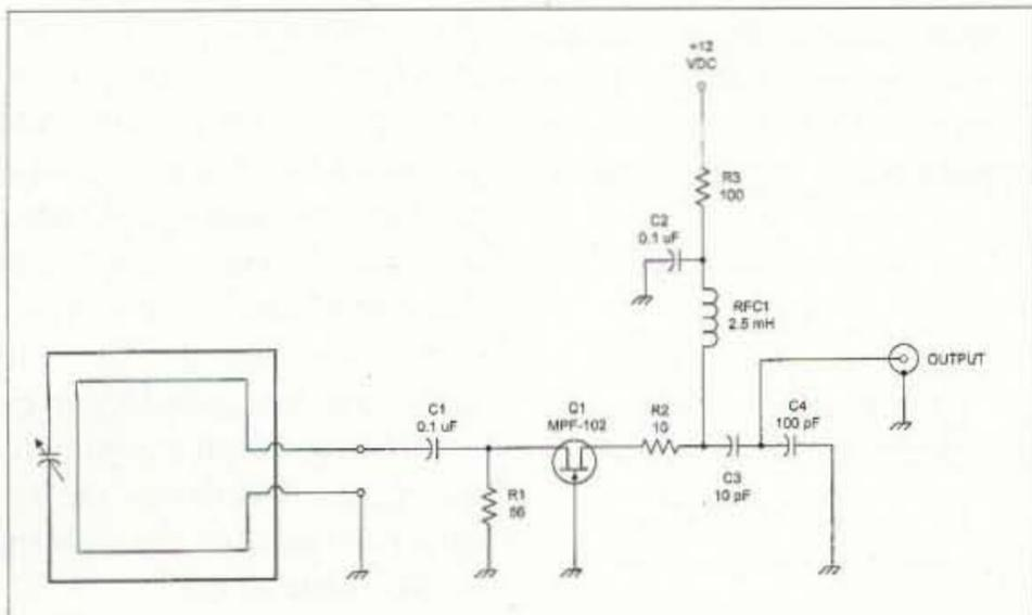
Fig. 9. Common gate JFET preamplifier.
