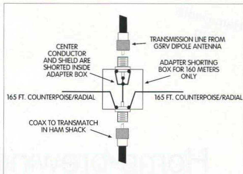
**Fig. 1.** Details of the adapter shorting box and counterpoise/radial hookup used at the base of AD1B's G5RV dipole antenna to permit him to temporarily utilize the antenna on 160 meters as a top-loaded vertical.
