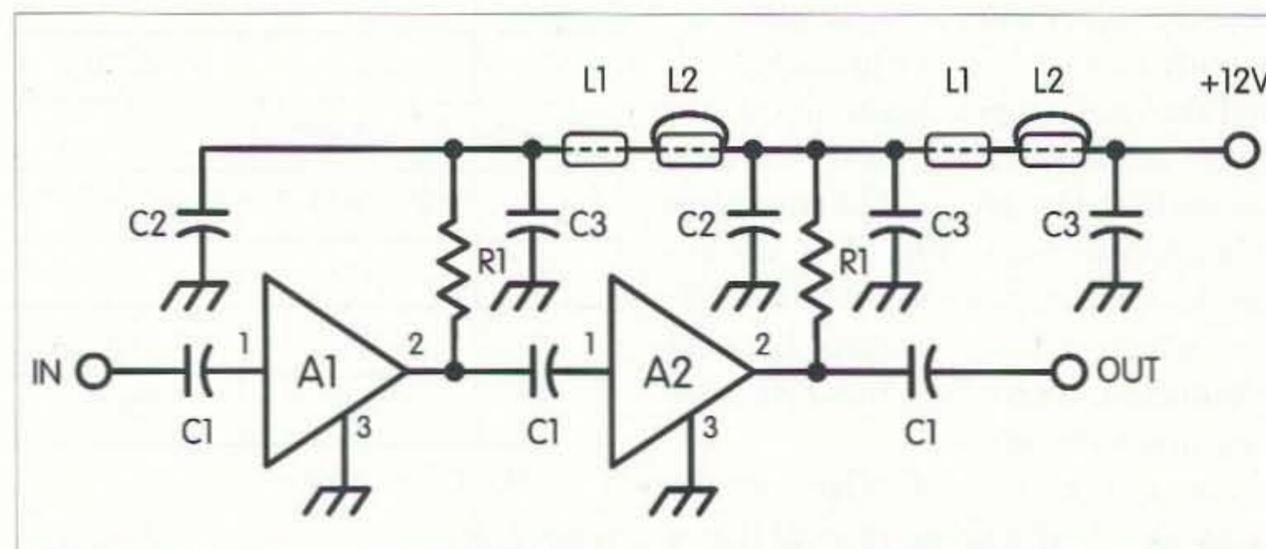
Fig. 3. Two MWA110s produce a broadband preamp.
