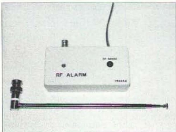
Photo C. The completed project and the telescopic antenna.
