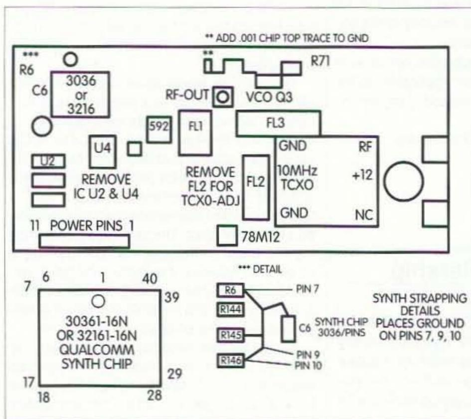
Fig. 1. Block diagram of the Qualcomm synthesizer board. Originally intended for operation near 800 MHz, it is converted to 1152 MHz for marker or local oscillator use. Board size is 5 by 9-1/4 inches. It sports a high-accuracy onboard 10 MHz TCXO.
