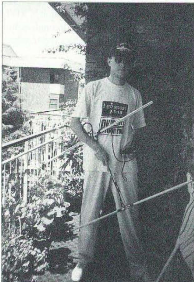
**Photo A.** The author, ready for the RDF challenge: handie-talkie in one hand, two-element phased beam antenna in the other.
