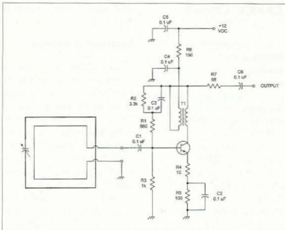
Fig. 6. Bipolar NPN transistor preamplifier.
