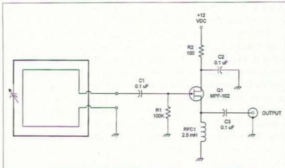
Fig. 10. Common source JFET preamplifier.
