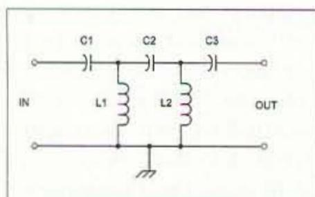
Fig. 14. High-pass filter.
