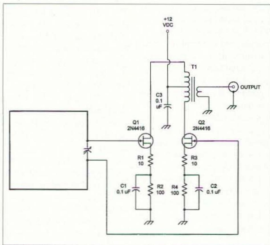
Fig. 12. Differential JFET preamplifier.
