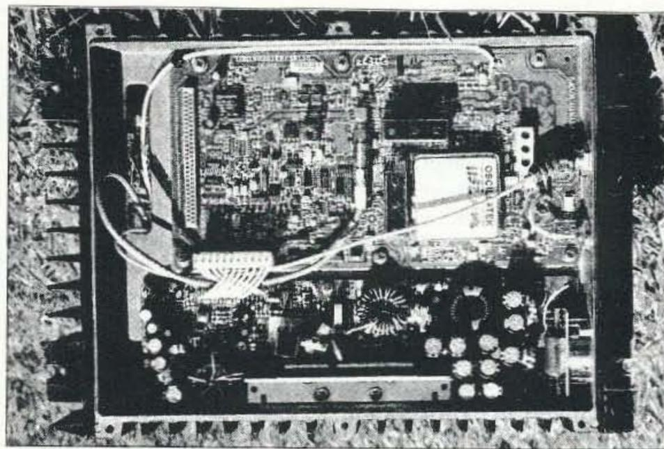
**Photo A.** Completed I296 transceiver using 1152 synth board. Unit power supply is at bottom and 1152 synthesizer above. 3036 synth chip at upper left. Large silver-colored unit near middle right is the high-precision 10 MHz TCXO. Synth PC board size is 5 by 9-1/4 inches.
