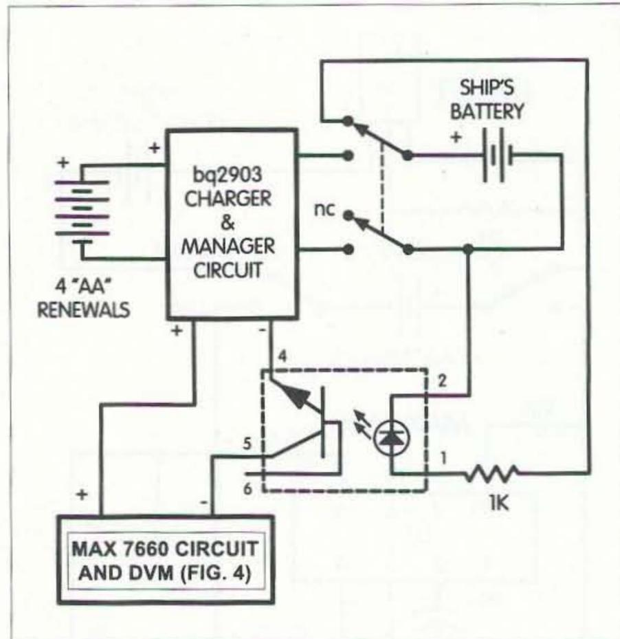
Fig. 7. Using an optoisolator and DPDT switch.
