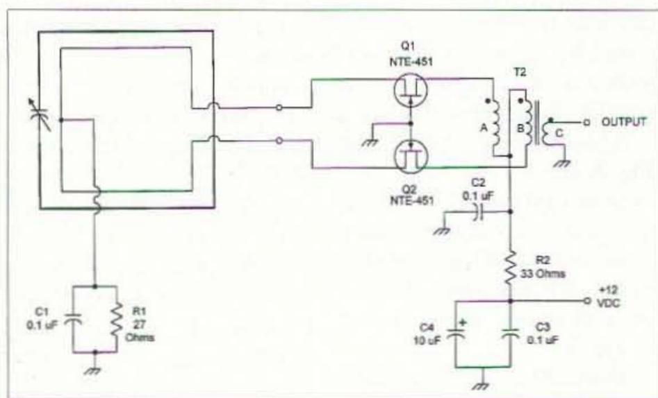
Fig. 11. Loop integrated push-pull preamplifier.
