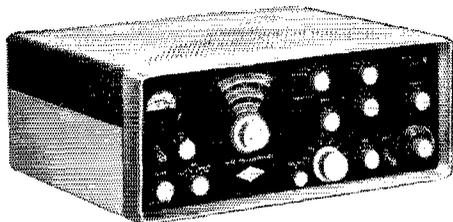
The Gonset G-76 with either the DC or AC power supply is capable of operating on low or high power—from 20 watts to 100 watts AM phone and 20 to 120 watts C.W. The power supplies include all necessary cables for fixed station or mobile installation.
