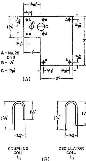
Fig. 2—(A) Details of the Plexiglas or polystyrene sheet that supports the components. (B) Dimensions of coils L<sub>1</sub> and L<sub>2</sub>. The material is No. 12 tinned copper wire.
