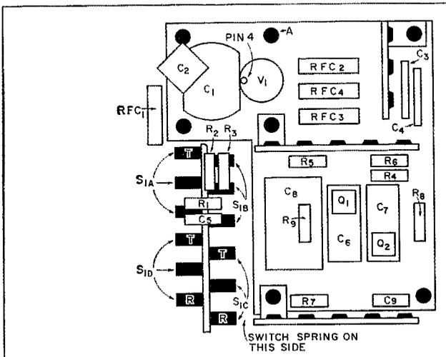
Fig. 3—Location of components on the clear plastic sheet. One 3-terminal and two 5-terminal tie-point strips are required.
