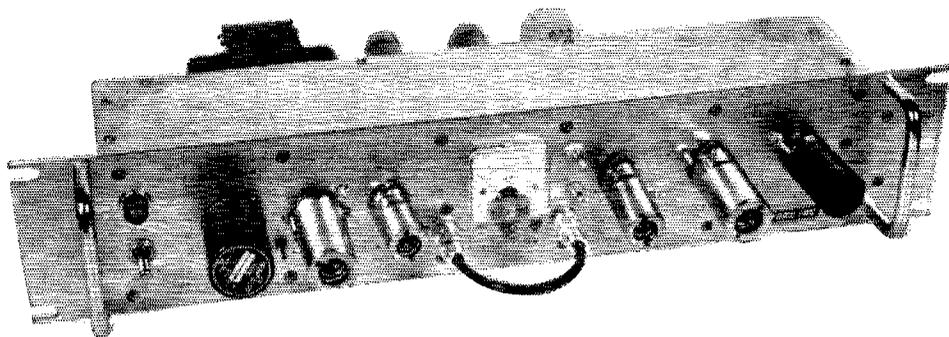
The Model 100 converter for fixed frequency commercial and military applications anywhere from 20 to 200 mc. This unit uses the 417A for the best possible noise figure, and includes a regulated power supply. Rack panel, 3 1/2" high. Also available is the 100A for 200-500 mc. This uses the latest nuvistor type 8058 in a two stage RF amplifier.
