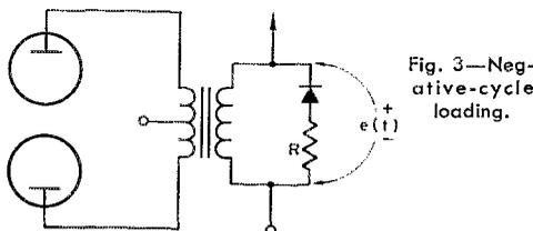
Fig. 3—Negative-cycle loading.
