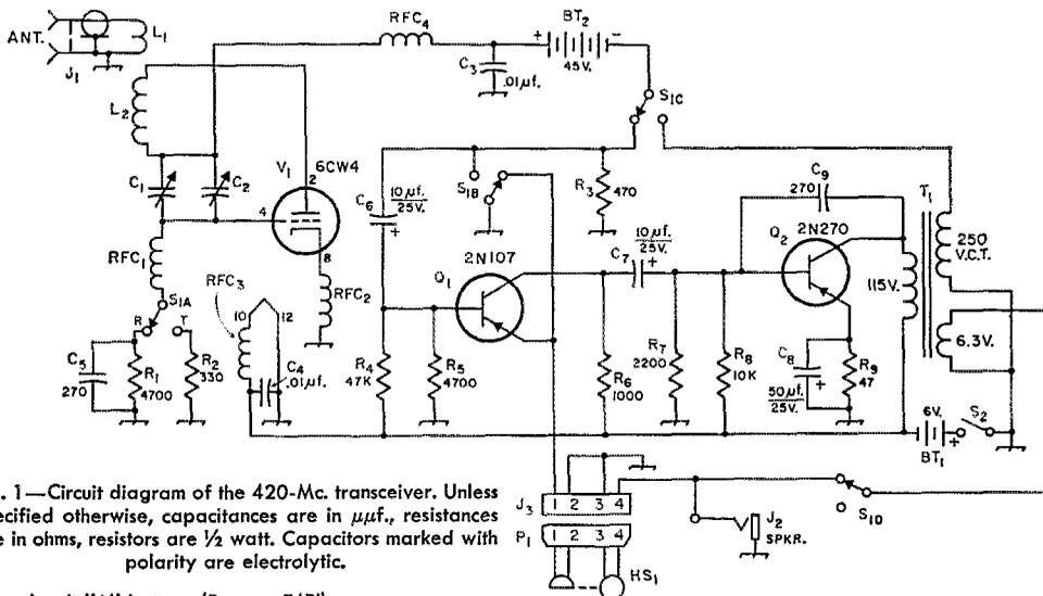
Fig. 1—Circuit diagram of the 420-Mc. transceiver. Unless specified otherwise, capacitances are in  $\mu\text{mf.}$ , resistances are in ohms, resistors are  $\frac{1}{2}$  watt. Capacitors marked with polarity are electrolytic.
