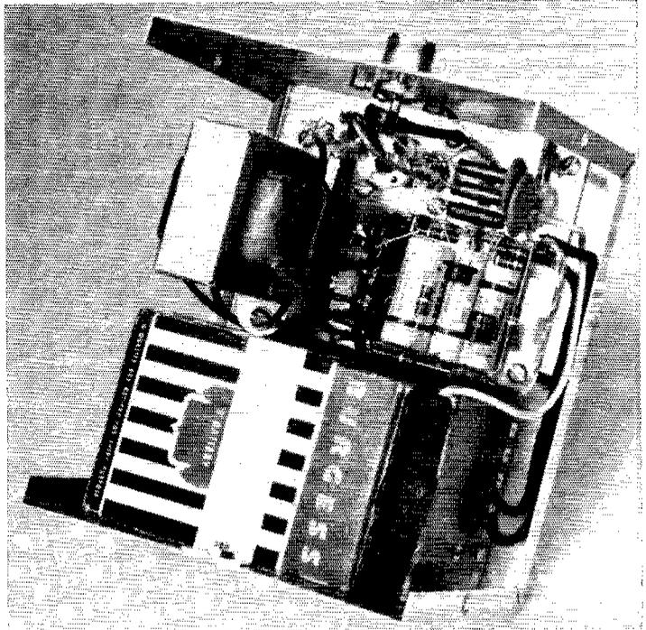
from a  $7 \times \frac{3}{4}$ -inch piece of scrap aluminum to secure the batteries to the lower half of the Minibox. Mount the send-receive switch,  $S_1$ , just above the strap, bolting it to the chassis with the same screw that holds the end of the strap. The switch spring should be on the right side as indicated in Fig. 3. Solder  $R_2$ ,  $R_3$ ,  $R_1$ , and  $C_5$  on the appropriate switch contacts.
