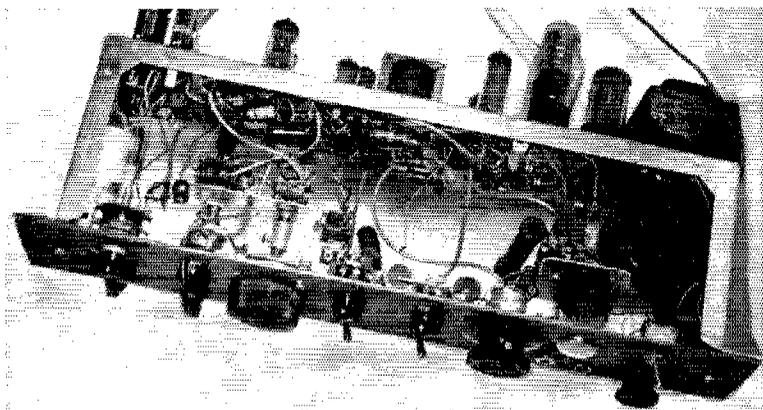
Front-bottom view. Panel controls, left to right, are for  $S_1$  (above) and  $R_7$  (below),  $R_1$  and  $S_2$ ,  $R_5$ ,  $R_2$  and  $S_3$ ,  $R_3$  and  $S_5$ ,  $R_3$ ,  $S_4$  and  $R_4$ . To the left of the latter are the 6AL7GT (mounted on a sub-panel) and the two headphone jacks  $J_3$  and  $J_4$ .
