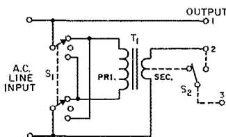
Fig. 2—Some adjustment of line voltage may be obtained by connecting a filament transformer so as to aid or buck the line voltage.  $T_1$  is a 5- or 6.3-volt filament transformer (10 amp. for a 1-kw. load).  $S_1$  is a two-pole three-position rotary switch (1 amp.). If the transformer has a center-tapped secondary, the addition of  $S_2$  shown in the dotted lines will permit a finer adjustment.  $S_2$  should be a s.p.d.f. toggle having a 10-amp. rating. See text.
