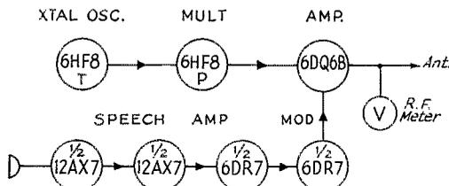
Fig. 1—Block diagram of the T-60 transmitter. Power supply, not shown, uses silicon rectifiers.
