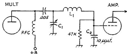
Fig. 2—Coupling circuit between multiplier and amplifier. The actual tuning capacitance for  $L_1$  is  $C_1$  in series with  $C_2$  (both have tube capacitances in parallel with them), plus stray capacitance.
