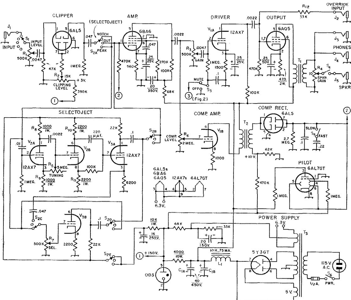
Fig. 1—Circuit of the versatile receiver-audio system. Unless indicated otherwise, capacitances are in  $\mu\text{f.}$  and resistors are  $\frac{1}{2}$  watt. Capacitors are paper or ceramic, excepting those marked with polarity, which are electrolytic. Resistances are in ohms.
