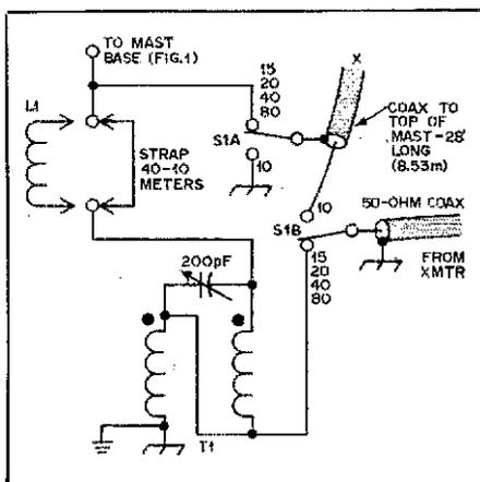
Fig. 2 - Schematic diagram of the base loading network. The connection to the mast base should be made with a short wire, no longer than one foot (0.3 m). The 200-pF capacitor should have a minimum of 1/16-inch plate spacing.
