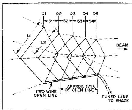
Fig. 2 — Spacing of the elements is indicated in this illustration. See text and Tables 1 and 2 for details.
