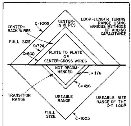
Fig. 5 — The chart shown above, providing dimensional guidelines for a single C-T loop, is based on the equation  $LF = C$ , where  $L$  is the outside dimension in feet,  $F$  is the frequency in MHz and  $C$  is a constant chosen for the size of the C-T loop to be constructed. Use the largest size possible for the best electrical results. This is particularly true when using C-T loop elements to form a parasitic beam.
