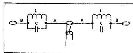
Fig. 2 — This drawing shows a typical multiband trap dipole. The lengths A-A can represent a half-wavelength antenna on 40 meters, while the overall B-A-A-B would be an 80-meter half-wavelength dipole.
