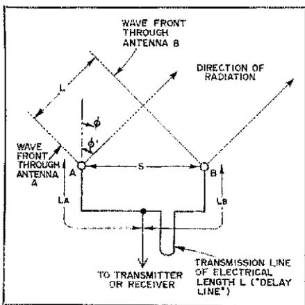
Fig. 1 — Two-element array with time-delay beam steering.
