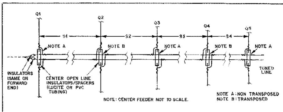
Fig. 3 — This illustration shows the physical arrangement of the internal transmission line of the QLP array.
