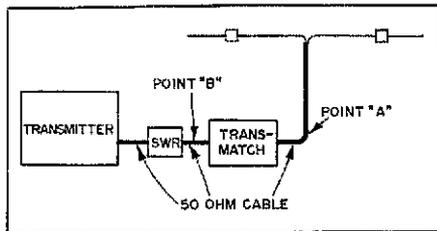
Fig. 3 — This drawing shows the correct placement of an SWR indicator when used for adjusting a Transmatch.
