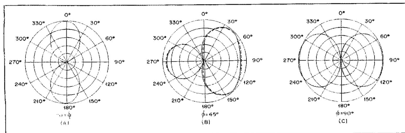
Fig. 4 — Azimuth patterns (linear voltage plots) of an array of two quarter-wave vertical monopoles spaced  $1/2$  wavelength apart.
