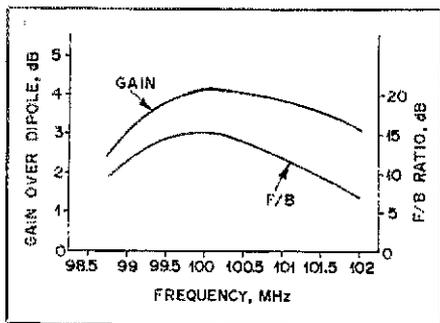
Fig. 1 — Curves depicting gain and FBR (front-to-back ratio) vs. frequency when the Yagi antenna is tuned for operation at 100 MHz.
