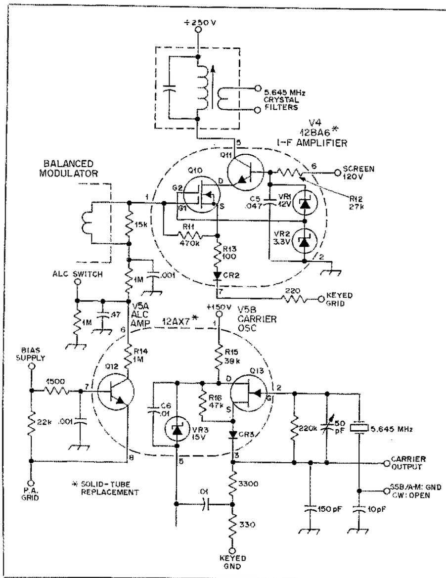
Fig. 4 - Solid-tube transistorization of the Drake T-4XB transmitter alc i-f amplifier, alc amplifier and carrier oscillator. See note of Fig. 3.
