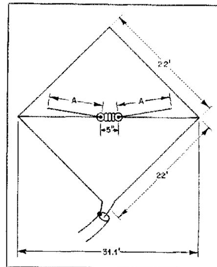
Fig. 3 — Dimensions for the 40-meter C-T quad are shown above. For the two-element beam the spacing between the driven element and the reflector is 20 feet. The length of the center-back wire (dimension A) is 12 feet, 9 inches for the reflector, and 9 feet, 11 inches for the driven element.
