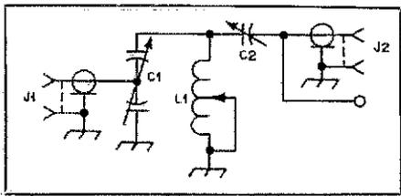
Fig. 1 — Circuit diagram of the Ultimate or Universal Transmatch. See text for details.
