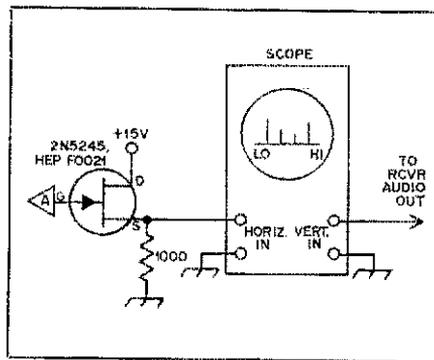
Fig. 2 — The sweeper may be connected to an oscilloscope as shown here. Signals within the passband of the receiver as it is scanned will appear as "pips" on the CRT. Sweep rate may have to be decreased in this application; see text for details.
