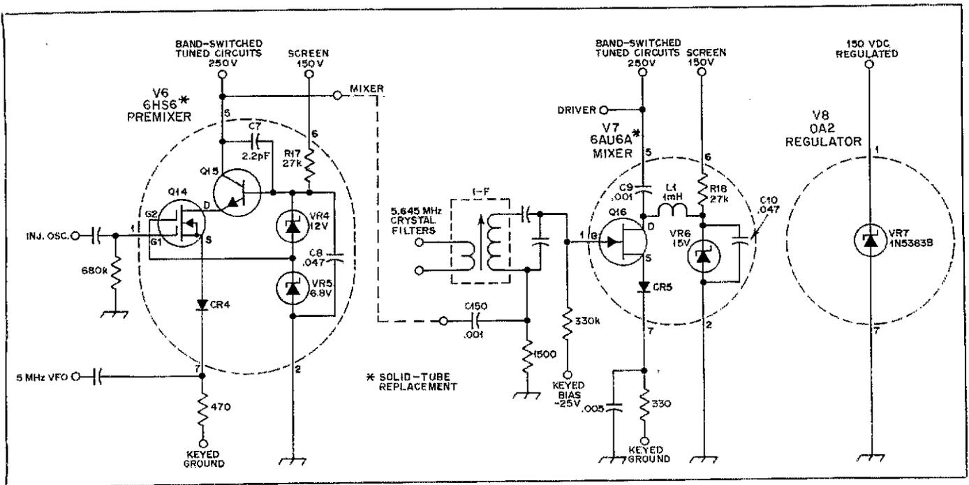
Fig. 5 — Solid-tubes for the Drake T-4XB pre-mixer, mixer and voltage-regulator vacuum tubes. See note of Fig. 3.
