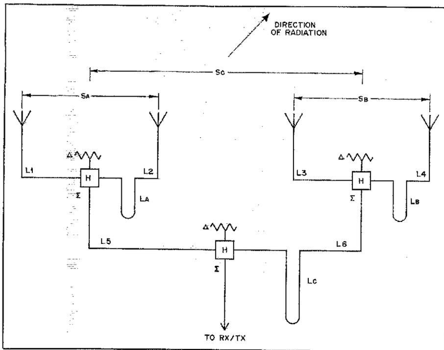
Fig. 5 — Configuration of a steerable four-element linear array. H denotes a ferrite hybrid power divider and matching transformer.  $\Delta$  denotes the difference port and  $\Sigma$  denotes the sum port.
