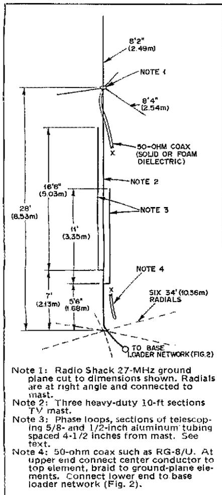
Fig. 1 - Details of the multiband radiating structure. See Table 1 for parts list. It is very important that a uniform spacing be maintained for the phasing loops, which may be supported at the bottom by shelf brackets. To support the upper portions of these loops, the author used homemade wooden spacers, 1/2 by 1 inch, which were soaked in paraffin and held in place by screws passing through the loop tubing and the main radiator tubing. Homemade Plexiglas spacers may also be used.
