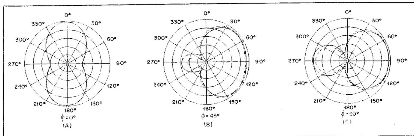
Fig. 3 — Azimuth patterns (linear voltage plots) of an array of two quarter-wave vertical monopoles spaced  $3/8$  wavelength apart.
