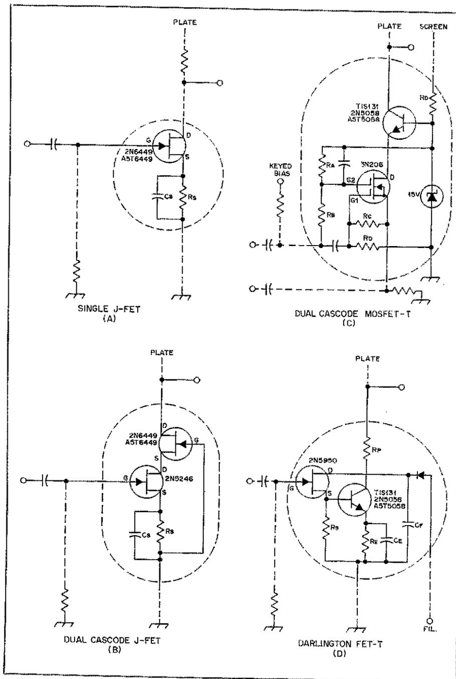
Fig. 2 — Four basic configurations are used to design solid-tube replacements for vacuum tubes. Dashed lines indicate equipment wiring. Specified  $R$  and  $C$  values depend on tubes being replaced. Solid-tube characteristics are given in Table 1.
