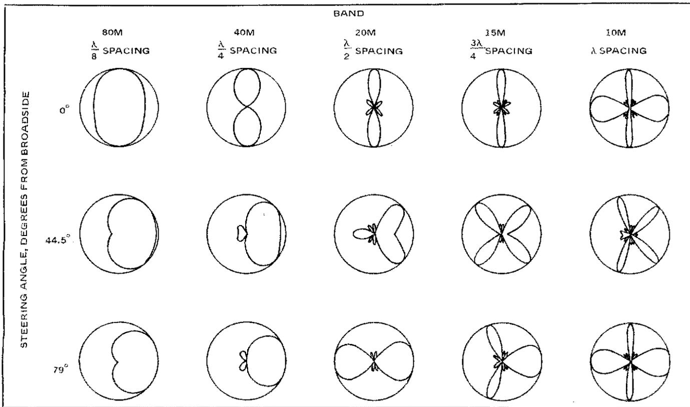
Fig. 7 — Idealized azimuth patterns for a five-band steerable four-element linear array of omnidirectional elements.
