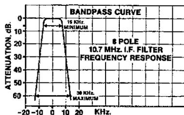
An 8-pole IF crystal filter greatly reduces adjacent channel interference.
