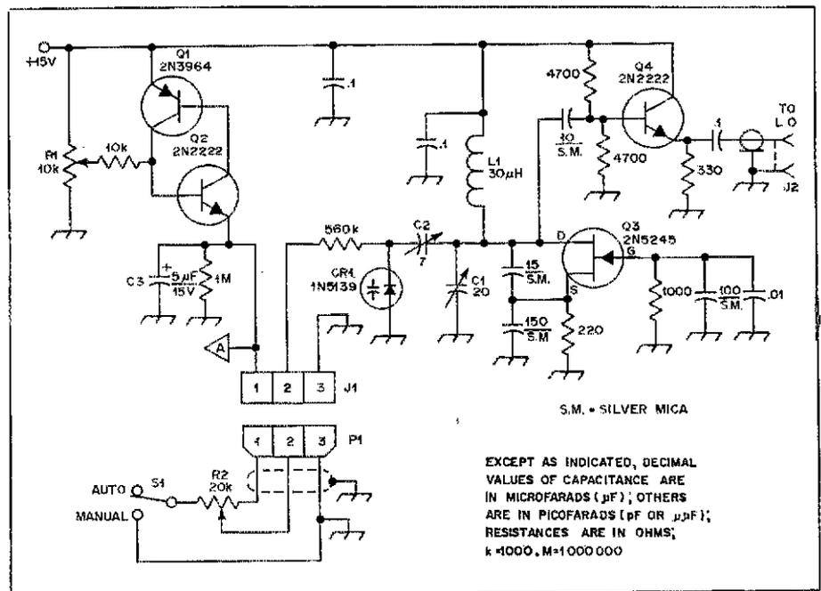
Fig. 1 — Schematic diagram of the sweeper circuit. The unit should be built in a metal enclosure, such as a Bud Minibox, for proper rf shielding. Capacitors are disk ceramic unless otherwise indicated. Resistors are 1/2 watt, 10-percent tolerance.
