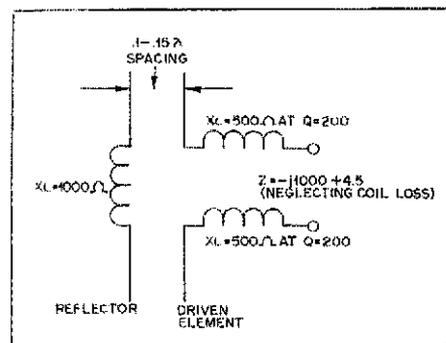
Taking into account the losses on loading coils of both the driven and
