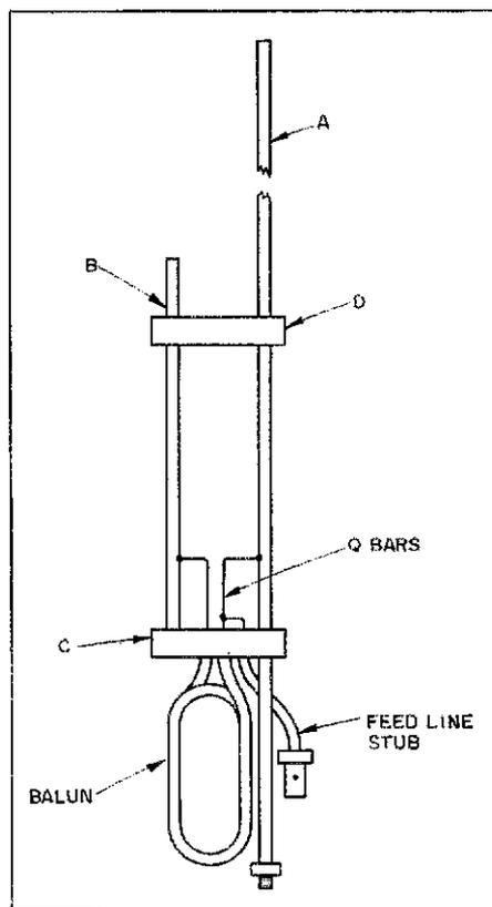
Fig. 1 — An overall view of the J antenna, showing the component parts. Dimensions are given in the text.
