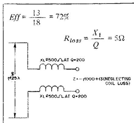
This means that 28 percent of the transmitting power applied to the antenna is dissipated in the loading coil. I have neglected any additional losses in the matching network which would result if the above antenna were driven by a 50-ohm source.
