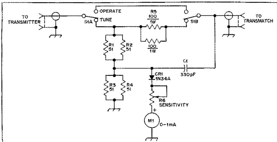
Protective circuit for QRP transmitters.
