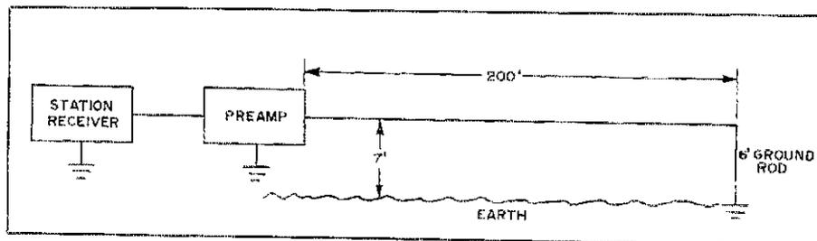
Fig. 2 — Details of the low-noise wire antenna used by the author with this preamp.
