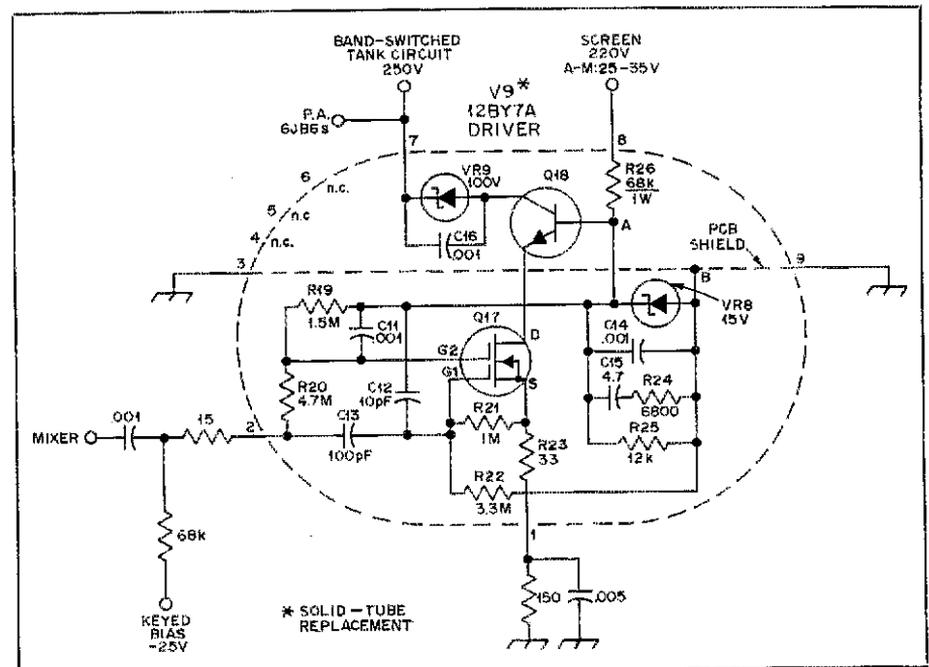
Fig. 6 — Solid-tube design for the Drake T-4XB power-amplifier driver:
