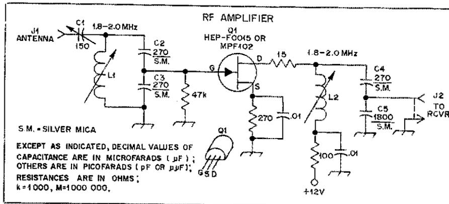
Fig. 1 — Schematic diagram of the 160-meter preamplifier. Fixed-value capacitors are disk ceramic unless otherwise indicated. Resistors are 1/4-W composition. C1 is an Arco 424 mica compression trimmer. For L1 and L2 see text. J1 is a binding post (insulated) and J2 is a phono jack.
