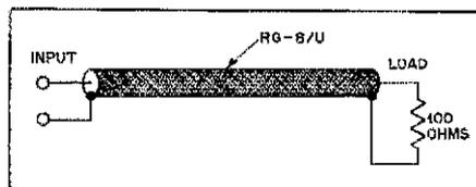
Fig. 2 — With 100 ohms connected at the load end of a length of RG-8/U, the problem is to determine what the line looks like at the input end.
