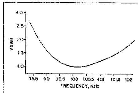
Fig. 2 — VSWR vs. frequency when the Yagi antenna is tuned for operation at 100 MHz.
